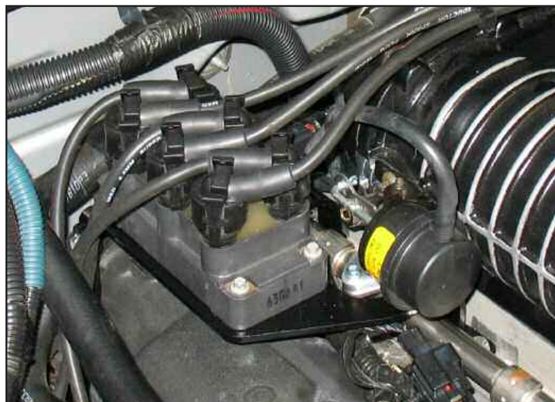
Figure AL coil installed
