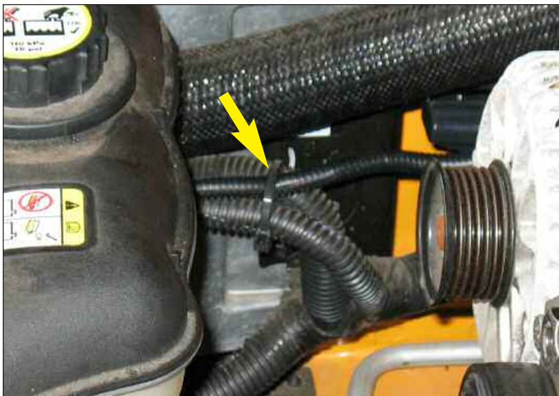
Figure HK secure harness
