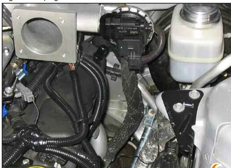
Figure AS EGR and tube
