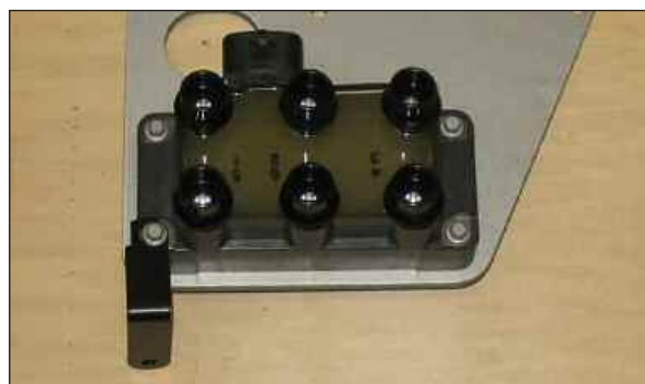
Figure AL1 coil plug wire bracket
