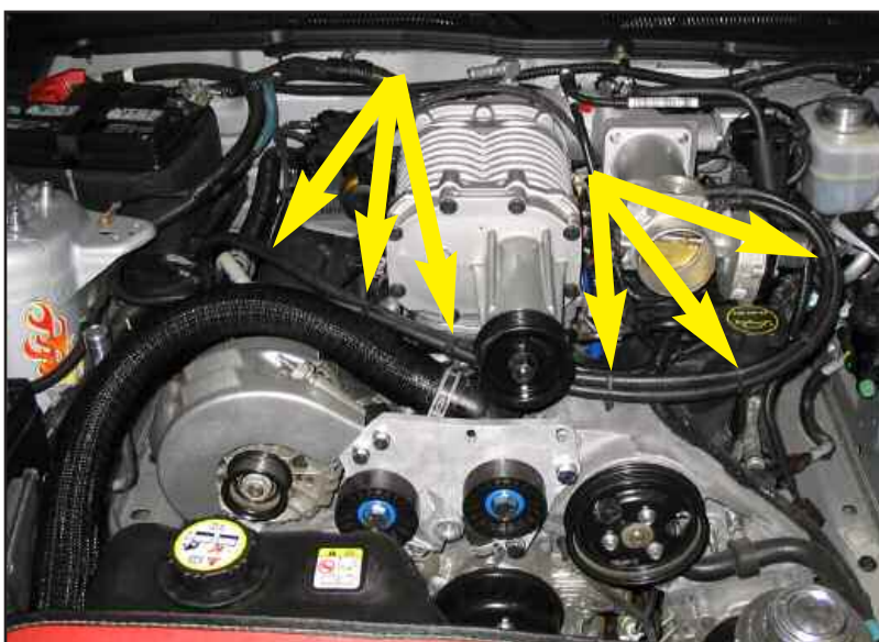
Figure AAC throttle body heater hoses (05 ONLY)
