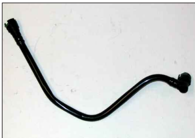
Figure BC complete new PCV tube
