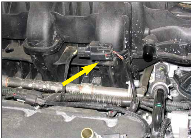
Figure H knock sensor connector
