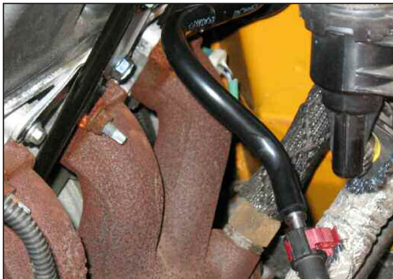
Figure RL connect fuel line
