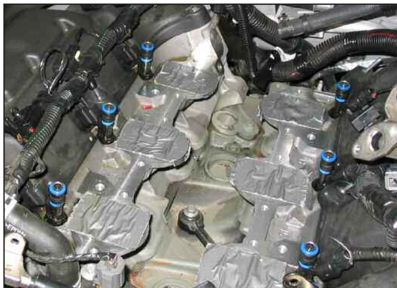
Figure IE injector orientation
