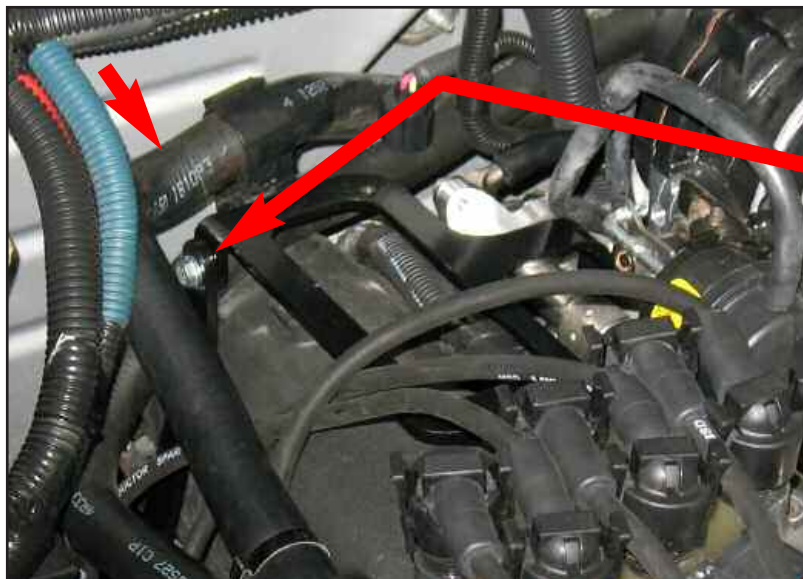
Figure AK coil bracket stay
