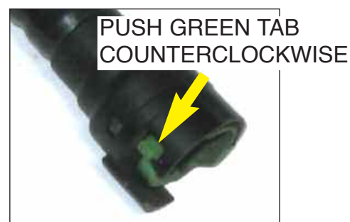
Figure D-1 hose connector
