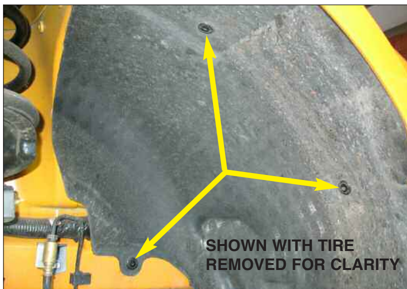
Figure ICD front inner fender rivets
