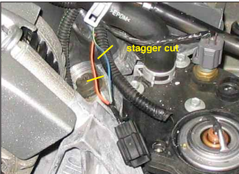
Figure HN harness tiewraps
