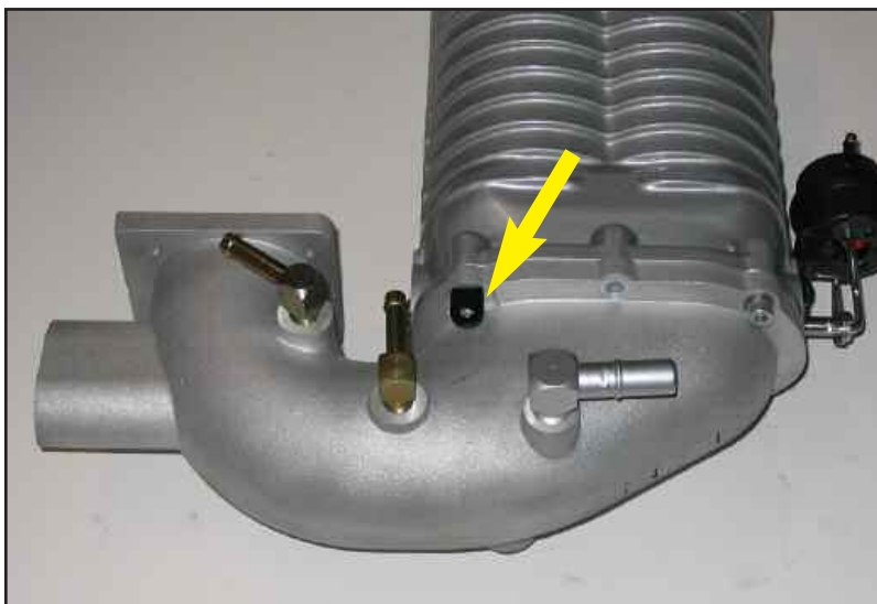
Figure SC install inlet adapter
