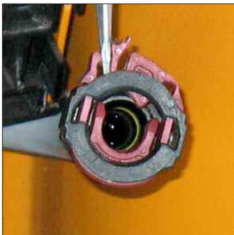
Figure IB-1 release red lock catch
