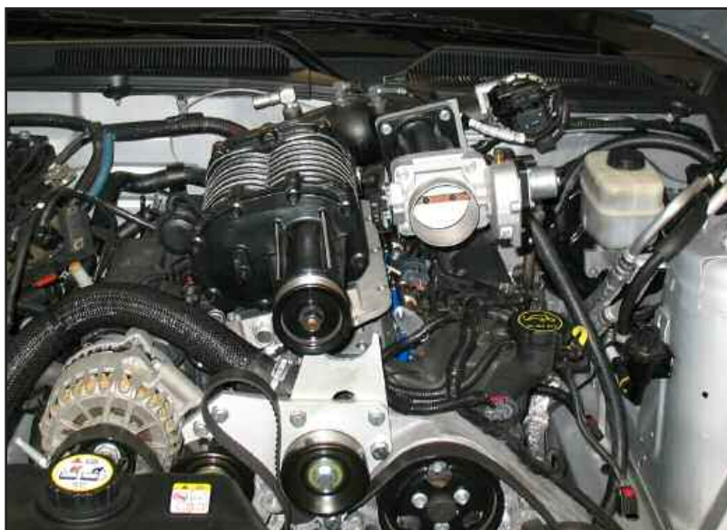
Figure AG install s/c assembly
