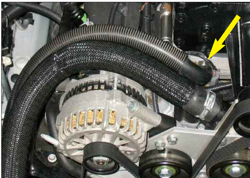
Figure ICAA inlet hose at ECU
