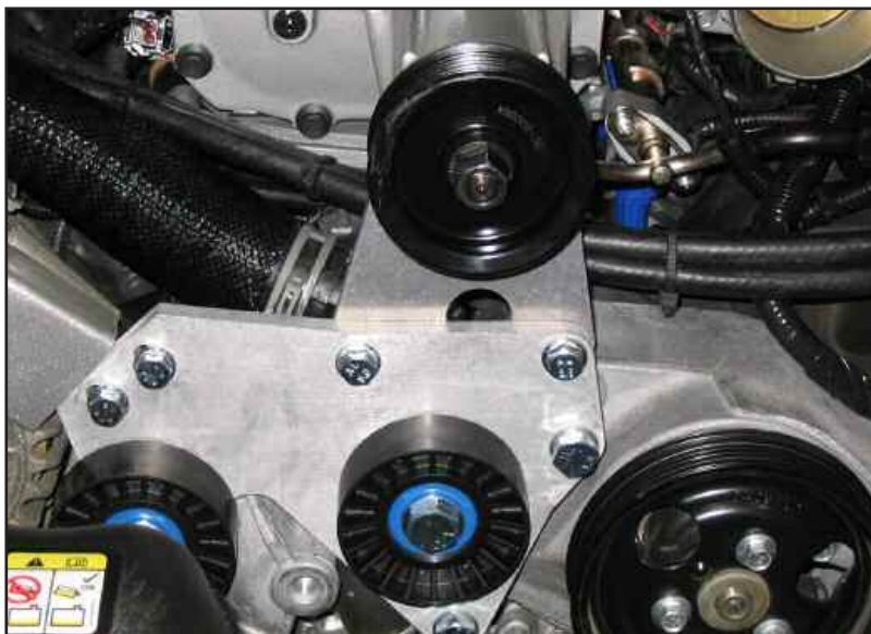
Figure AAF install nose support
