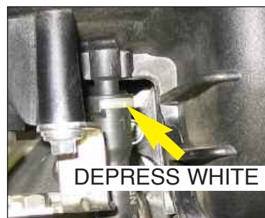
Figure O-2 vapor hose connector
