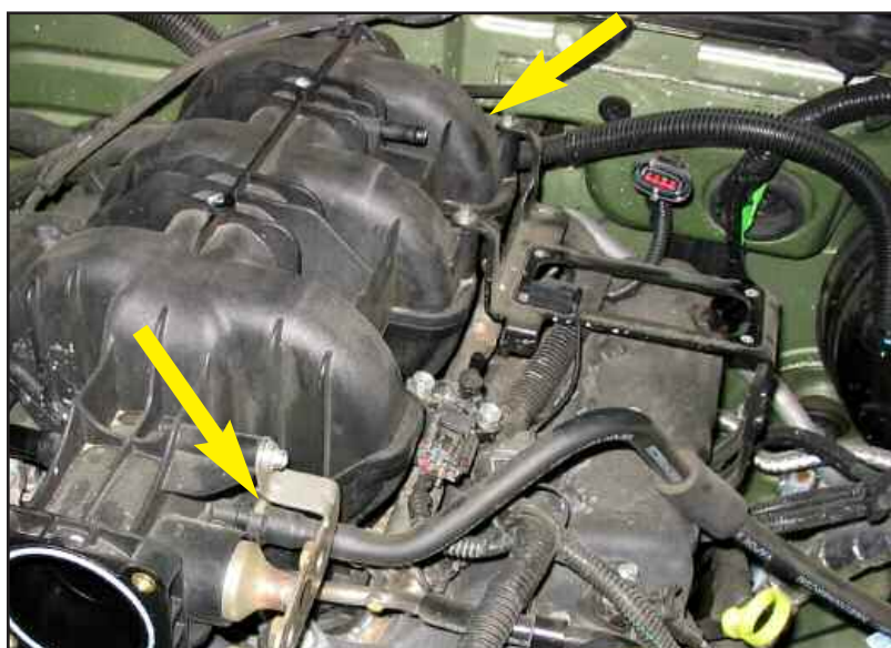
Figure O remove vapor and booster hoses
