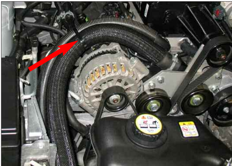
Figure ICAC inlet hose at ECU
