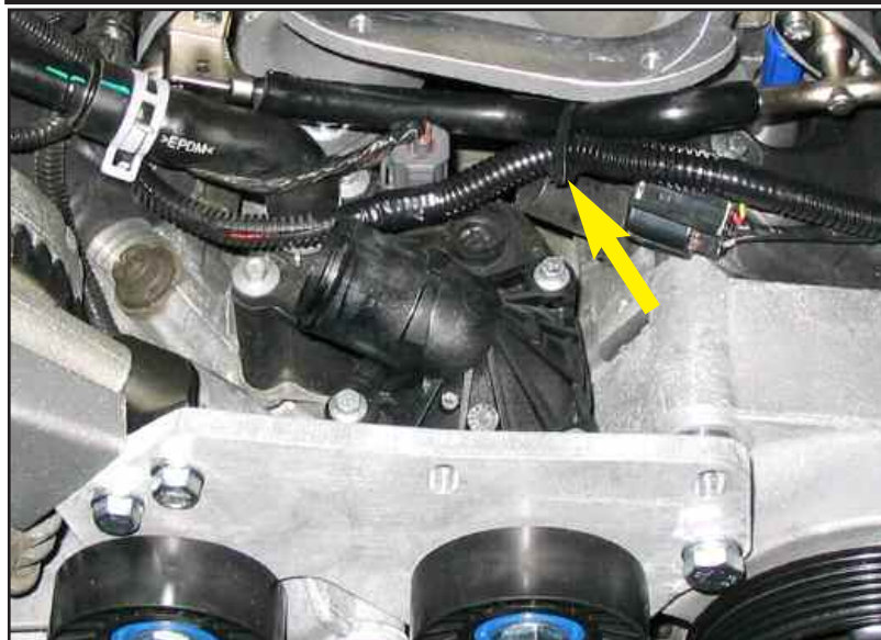
Figure AA install thermostat cover
