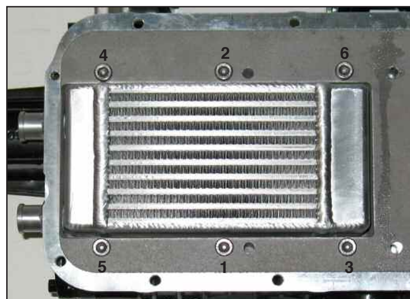
Figure SF install discharge manifold lid
