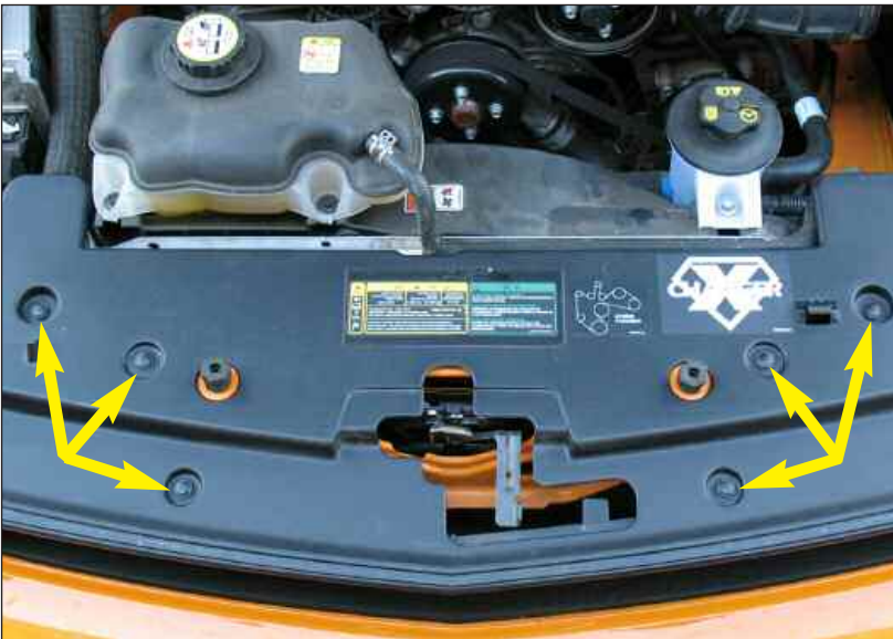
Figure ICA remove radiator cover
