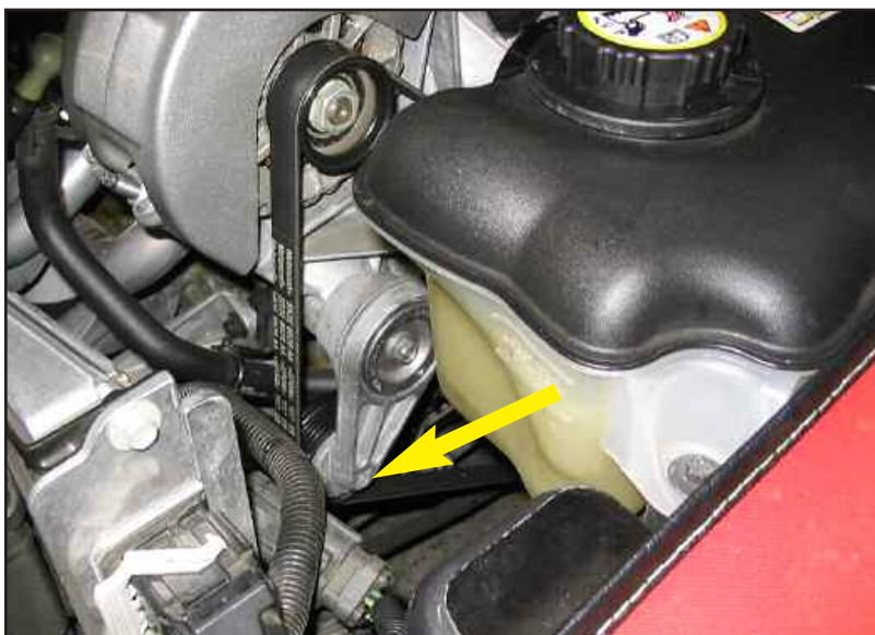
Figure U Remove drivebelt
