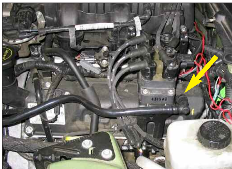
Figure I remove breather hose
