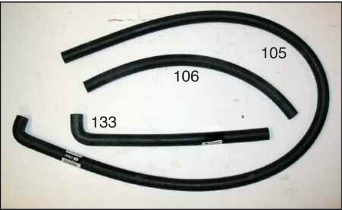
Figure PY intercooler hoses
