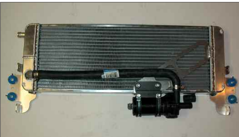
Figure ICS pump/hose installed
