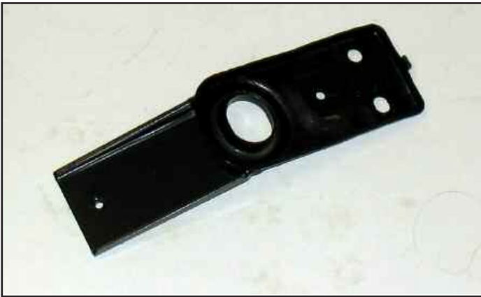
Figure PAD P/S reservoir bracket key no 132
