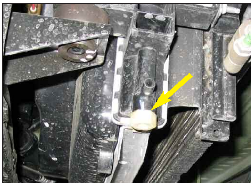
Figure C drain coolant
