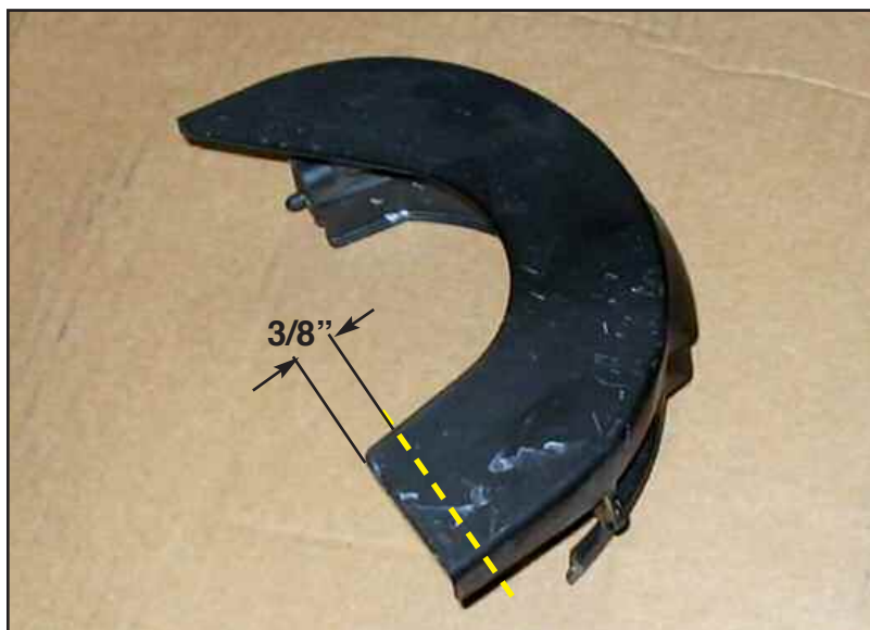
Figure W modify alternator cover
