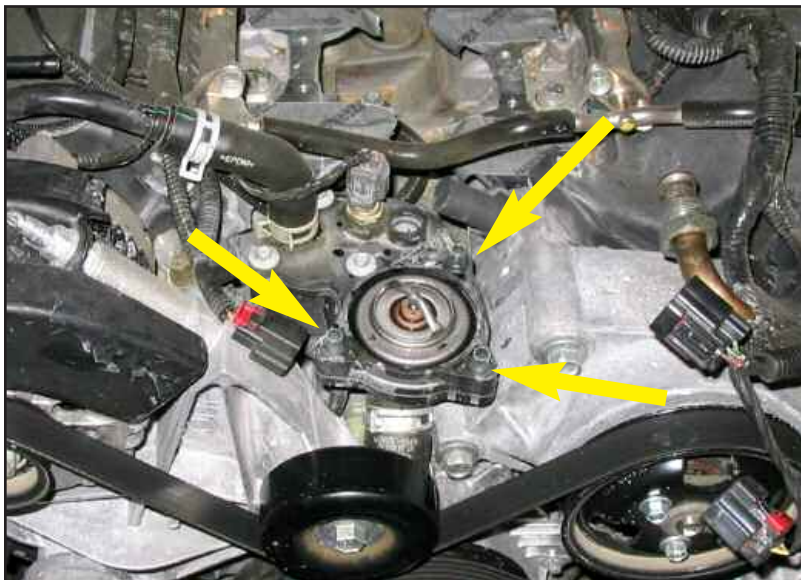
Figure T remove thermostat cover dowels
