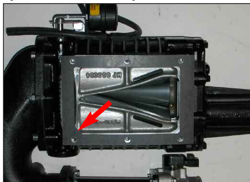
Figure SE discharge gasket
