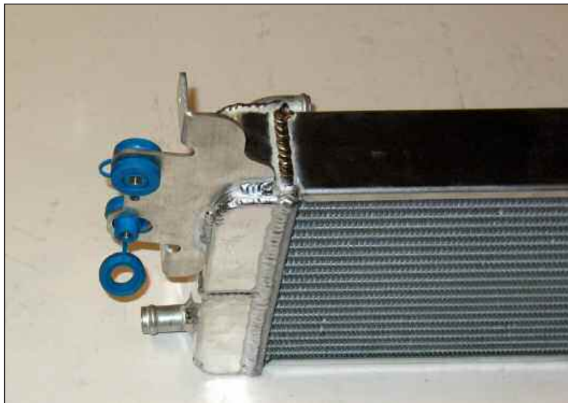
Figure ICR install exchanger isolators
