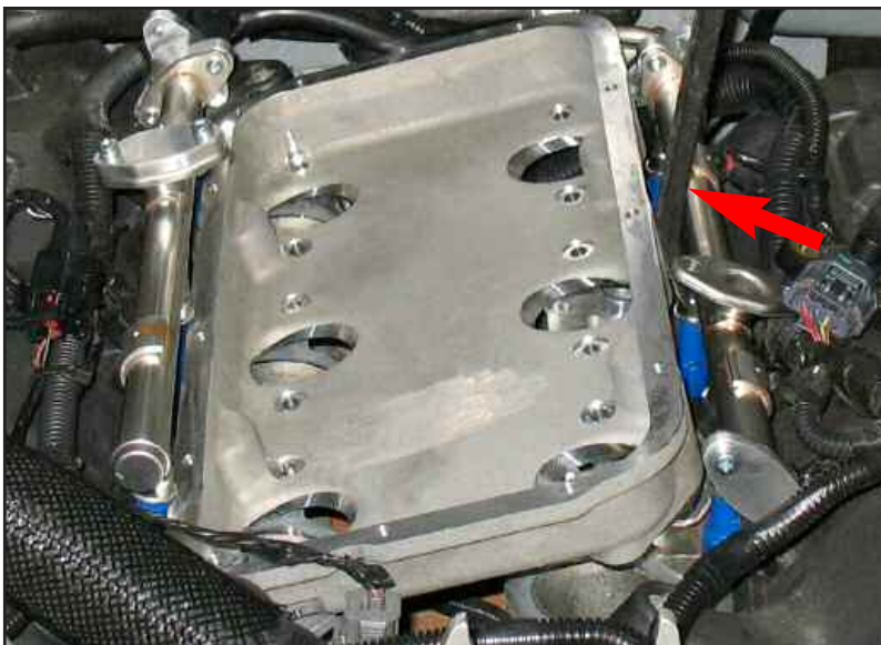
Figure AD discharge manifold installation
