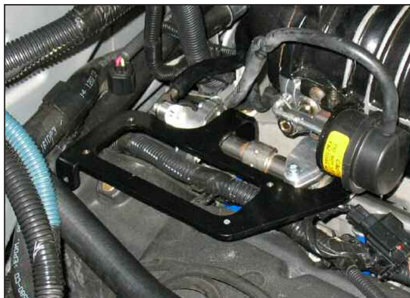
Figure AJ coil bracket
