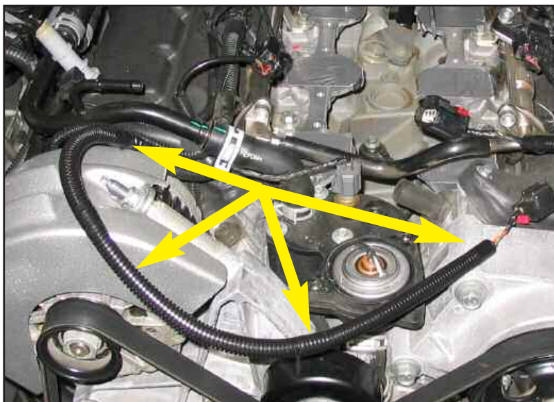
Figure HP install Throttle Actuator wire armor
