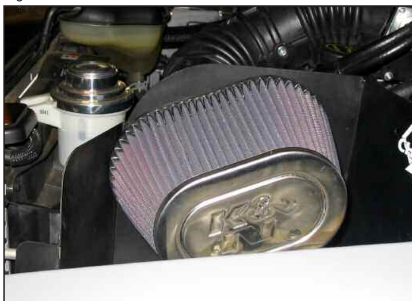
Figure ABO install air filter
