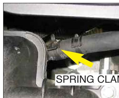
Figure O-1 brake booster connector
