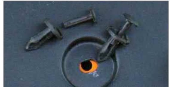
Figure ICB rivet detail
