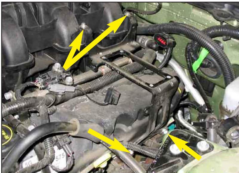
Figure N remove coil bracket
