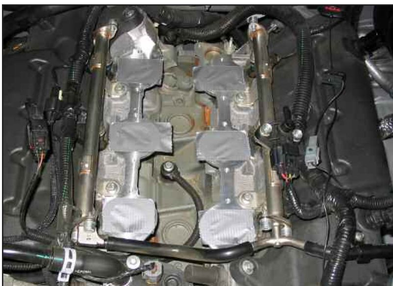
Figure R tape intake ports
