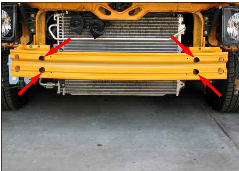
Figure ICO bumper support bolts
