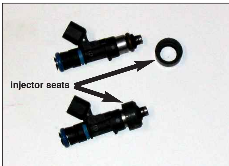
Figure IF injectors and seats
