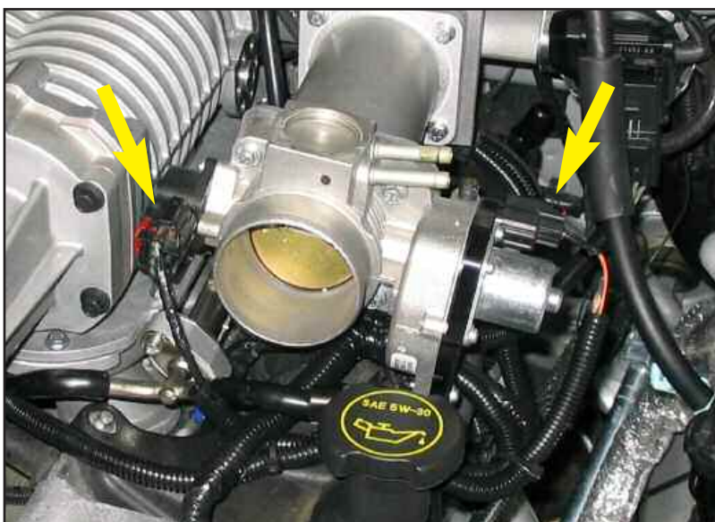
Figure AAB throttle body electrical connections
