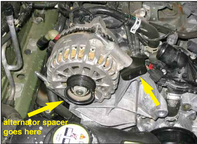
Figure DA install alternator spacer and bracket
