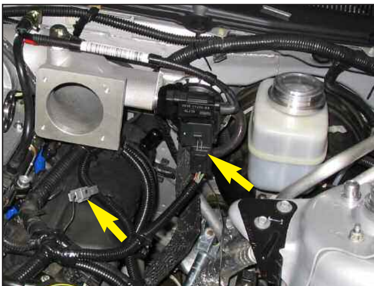
Figure AX vacuum source tube
