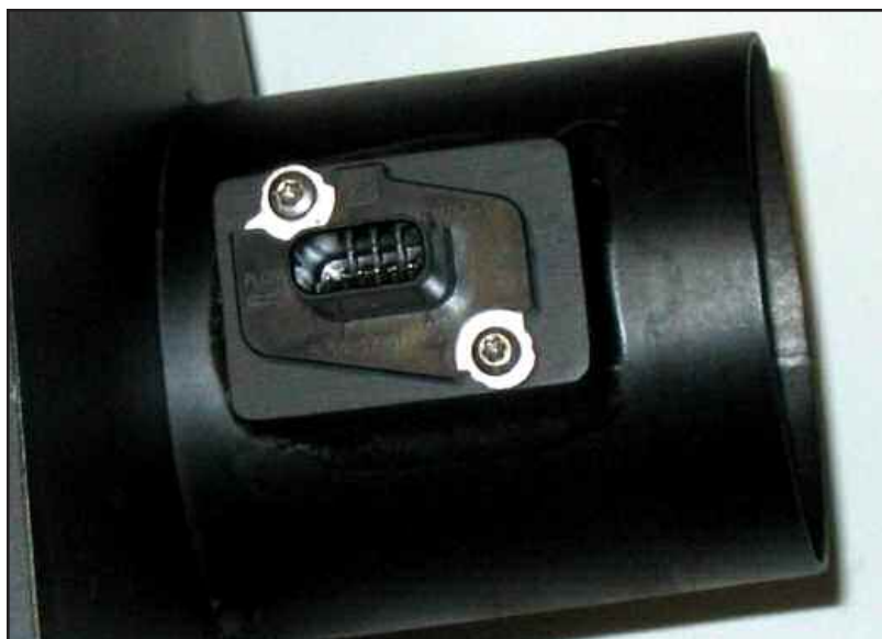
Figure ABH install MAF sensor
