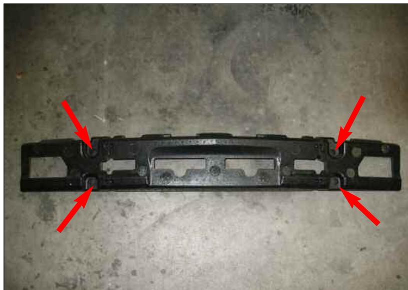
Figure ICM remove front bumper pad
