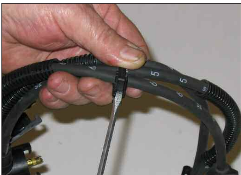
Figure AM remove plug wire retainers
