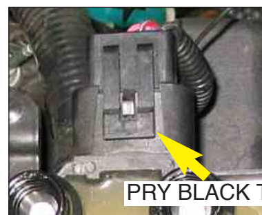
Figure M-1 coil connector
