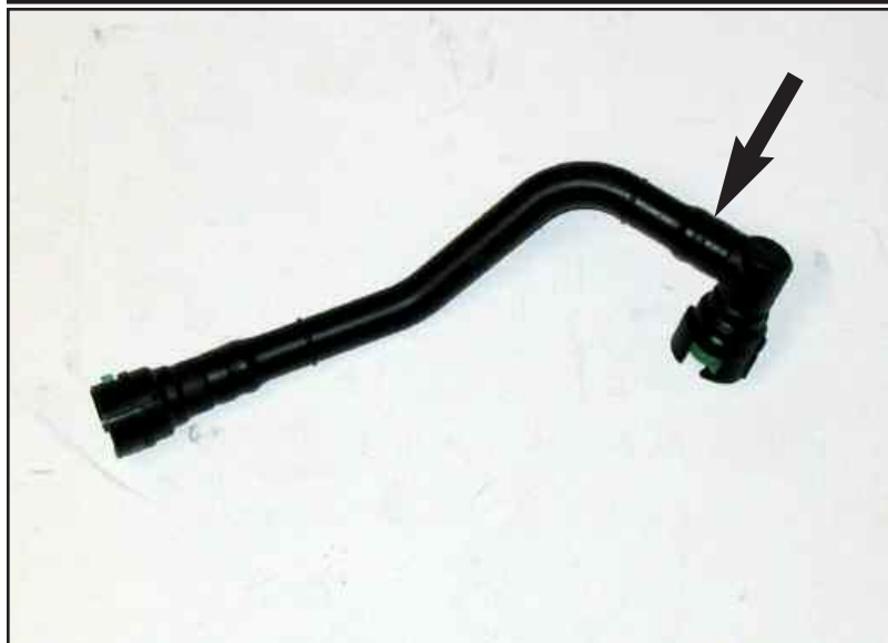
Figure BA remove PCV valve fitting
