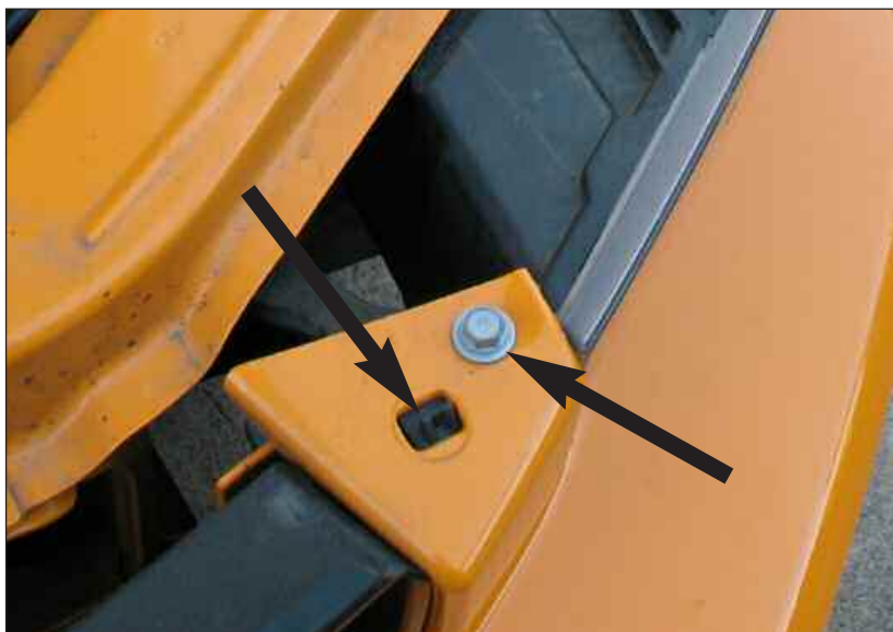
Figure ICI bumper cover upper bolt
