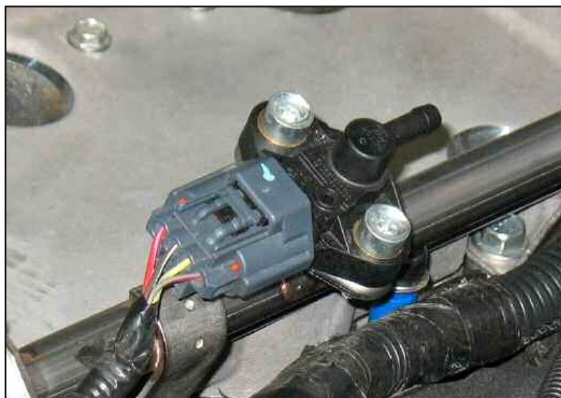
Figure AF fuel pressure sensor installed
