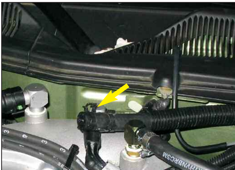
Figure AY brake booster hose
