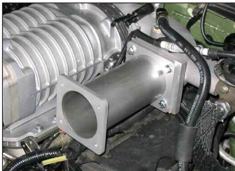
Figure AZ inlet extension
