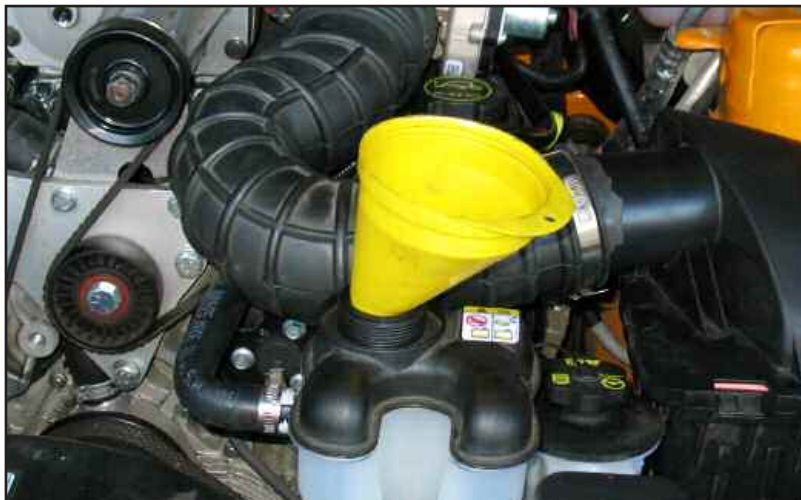
Figure HN fill surge tank
