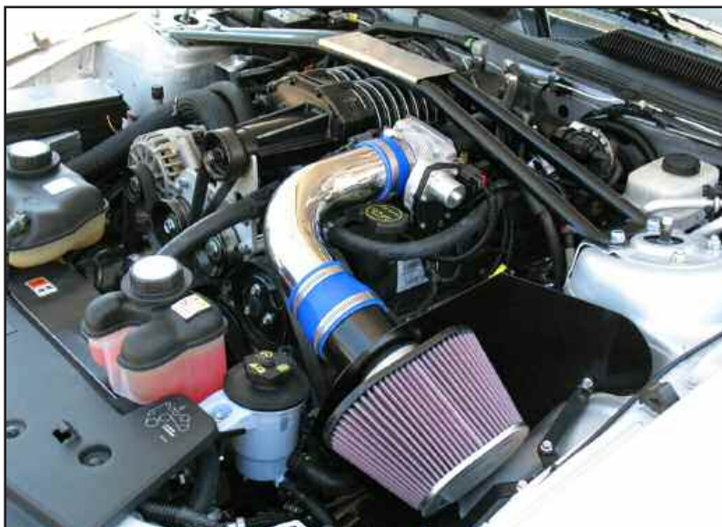
Figure ABM install inlet tube
