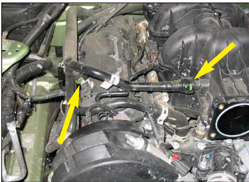
Figure G remove PCV tube
