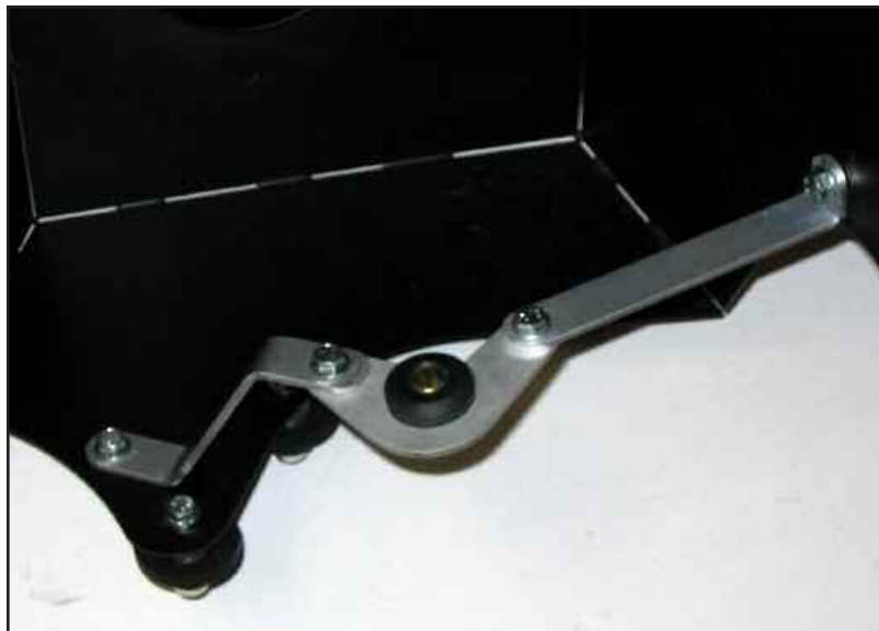
Figure ABF install airbox retainer
