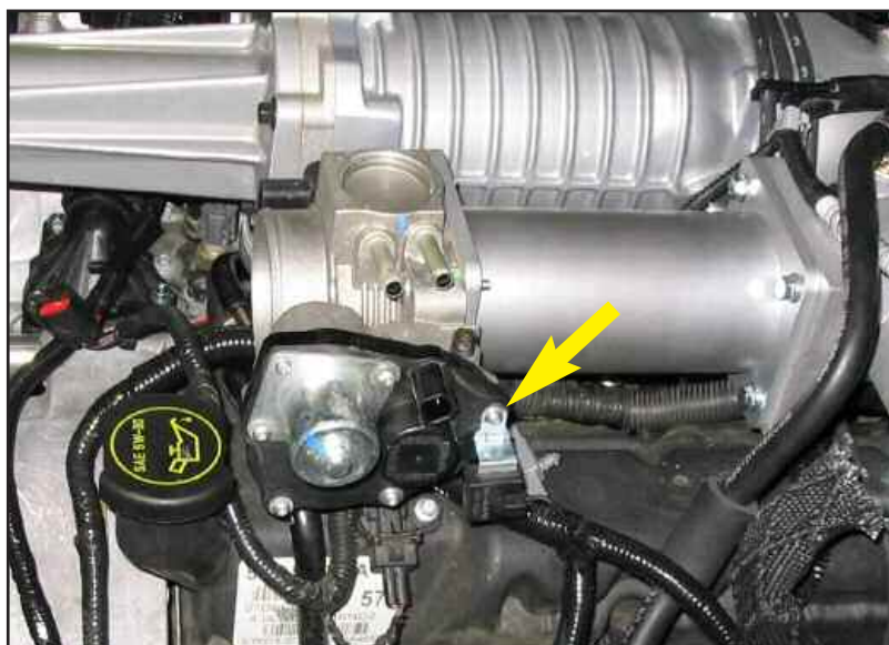
Figure AAA coil resistor
