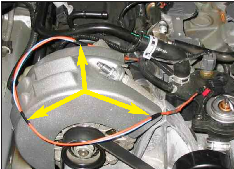
Figure HO tape Throttle Actuator wires
