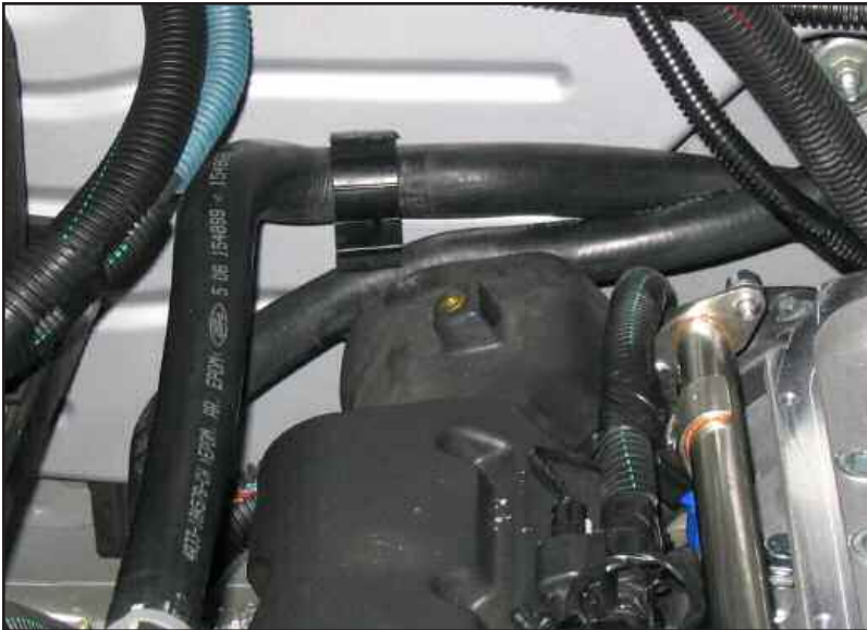
Figure AB position heater hoses
