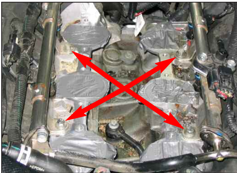
Figure ID fuel rail bolts
