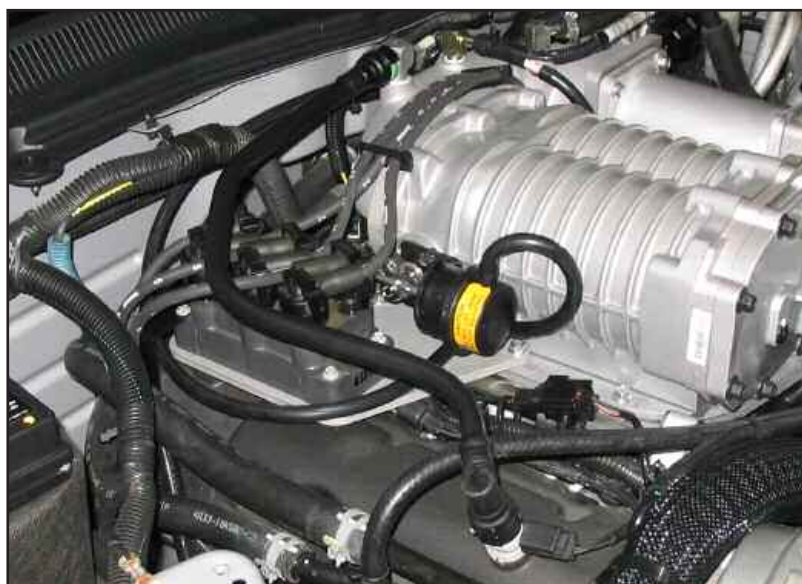
Figure AAH PCV tube installed
