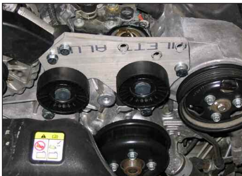
Figure DE install idler pulleys
