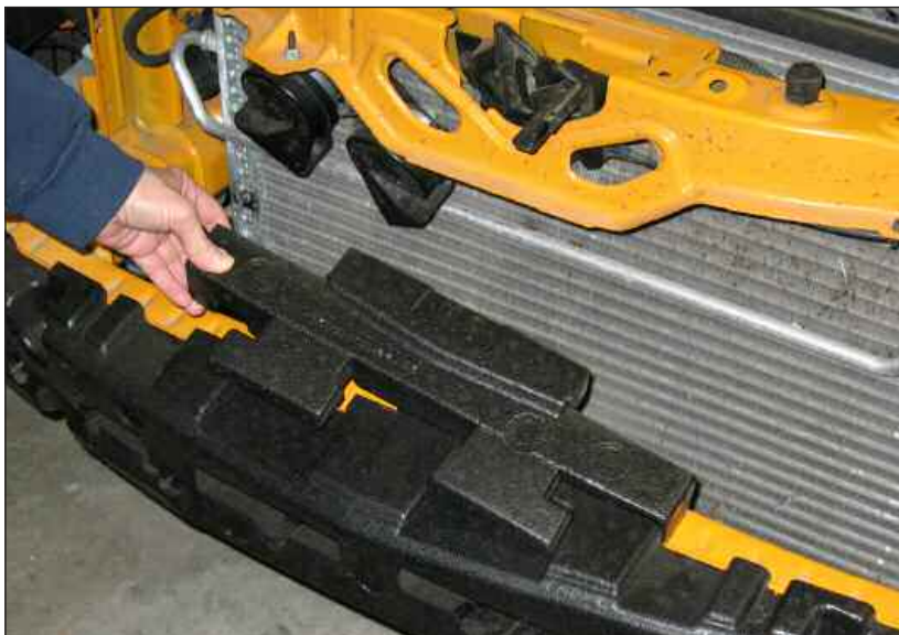
Figure ICL remove upper bumper pad
