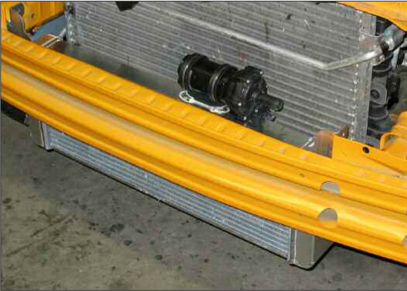
Figure ICU heat exchanger installed
