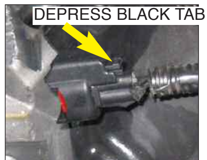
Figure IE-1 injector connector
