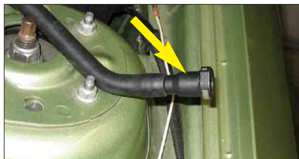
Figure AU remove hose connector
