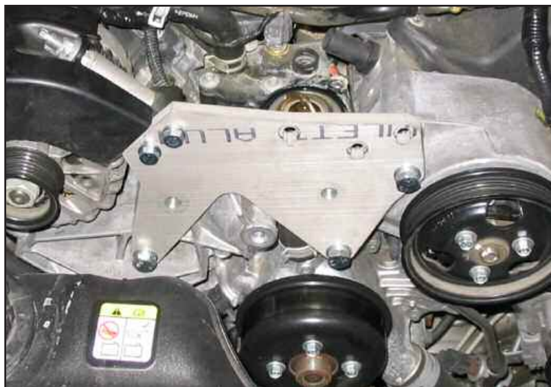
Figure DD install idler plate
