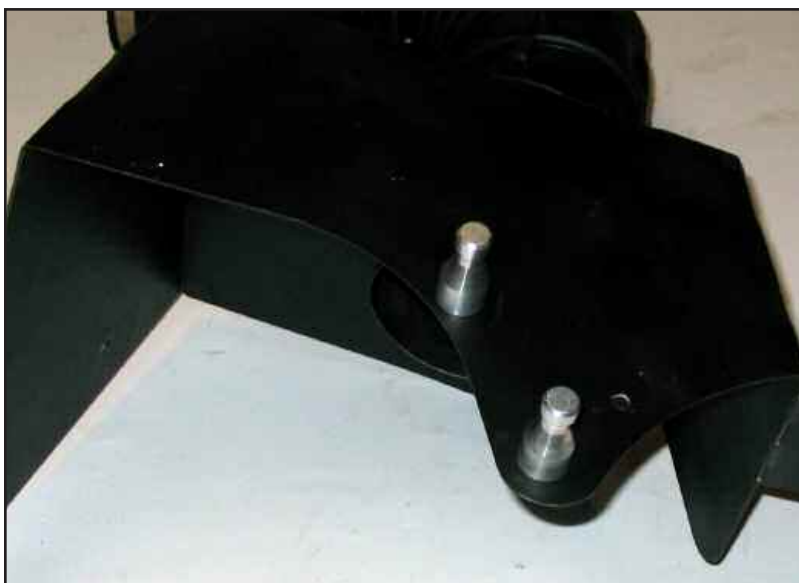
Figure ABE install airbox pins
