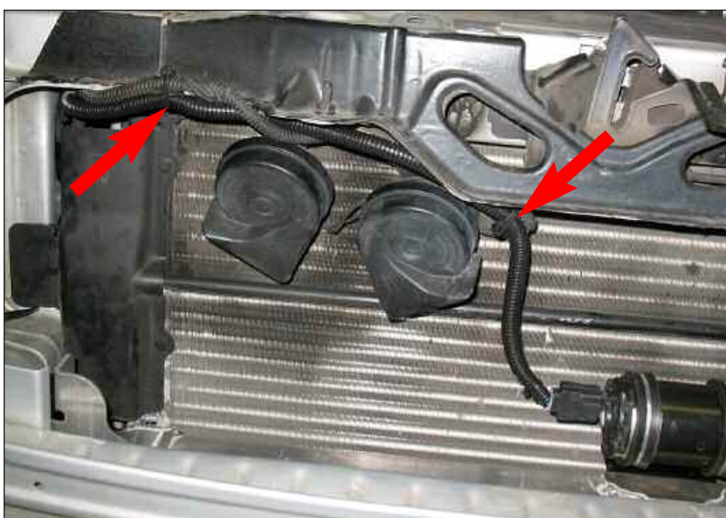
Figure HM harness routing
