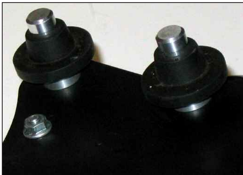
Figure ABG install airbox insulators
