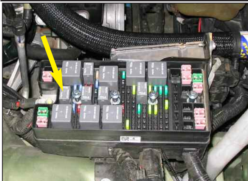
Figure A remove fuel pump relay
