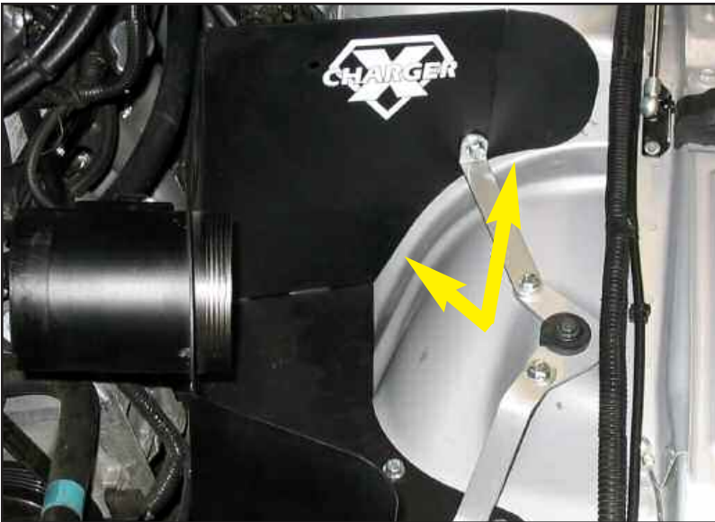
Figure ABJ install airbox
