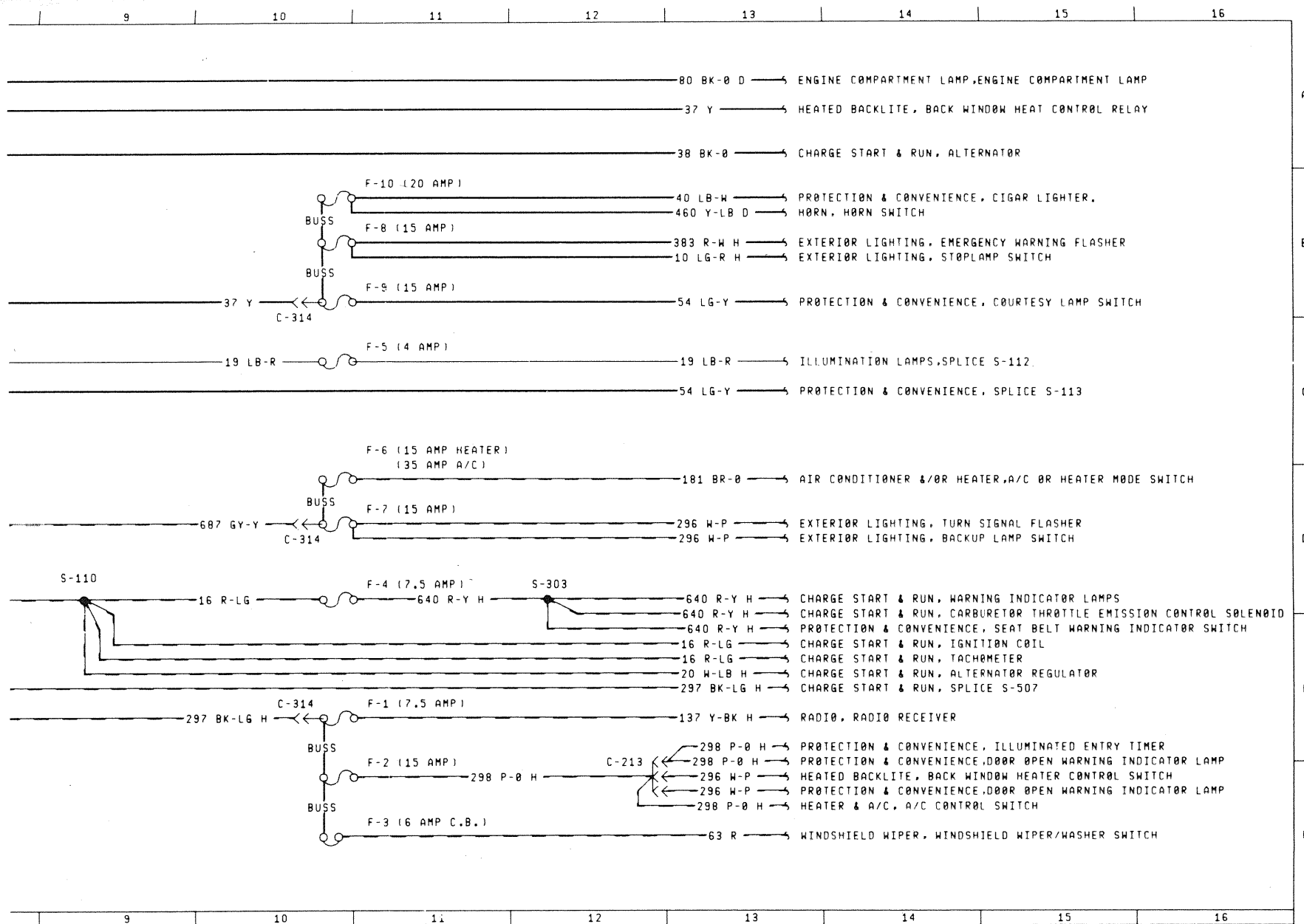
Fig. 13.140 (Cont'd) Wiring diagram, 1978 models: power distribution circuits. For color code see page 280
