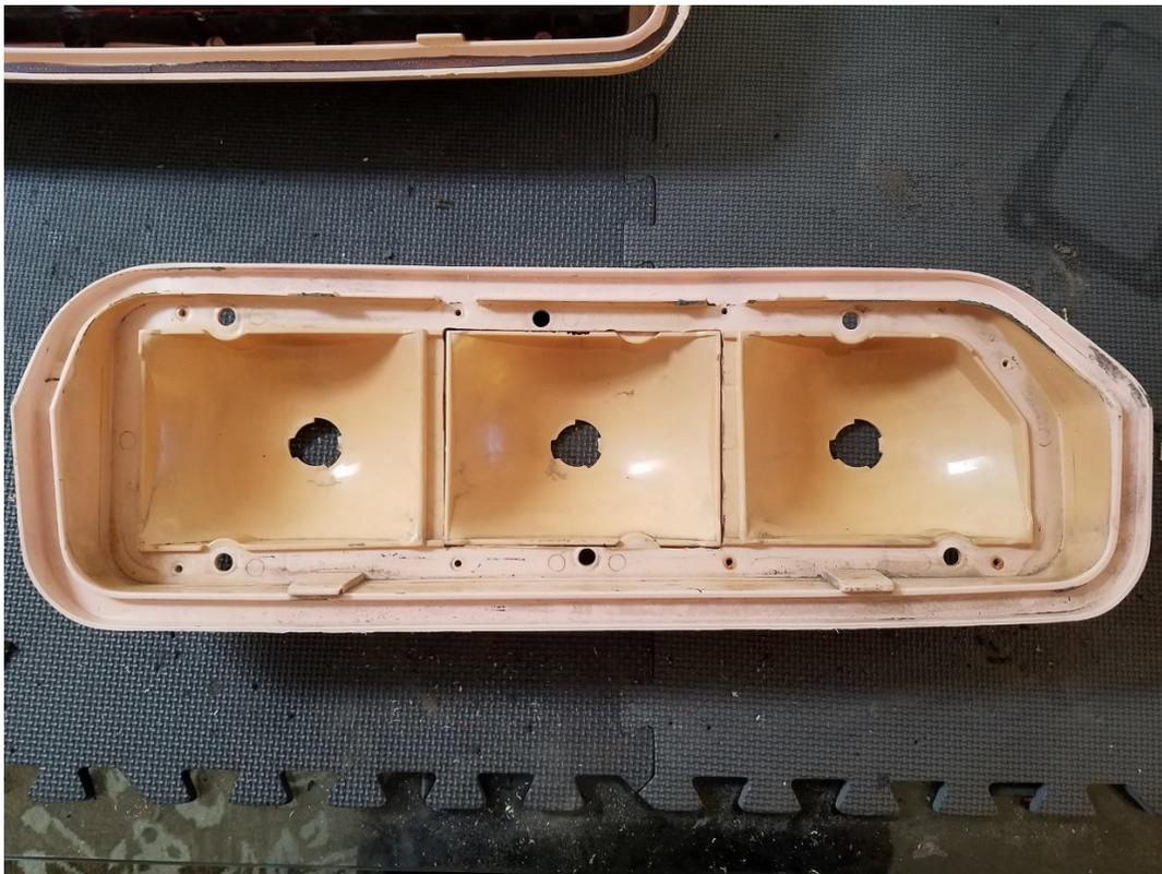
Once you've got your donor sections fitted properly, epoxy them into the lenses and housing. I have never been impressed with any kind of plastic epoxy. I used 3M Panel Bond to mate the donor sections. It's not cheap and it requires a special applicator gun, but this stuff is made to glue body panels together, and is about the strongest epoxy out there.
