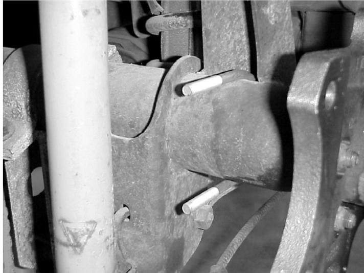
**STEP 25:** Slide the caliper brace into place over the U-bolt as shown and loosely install the nuts.
