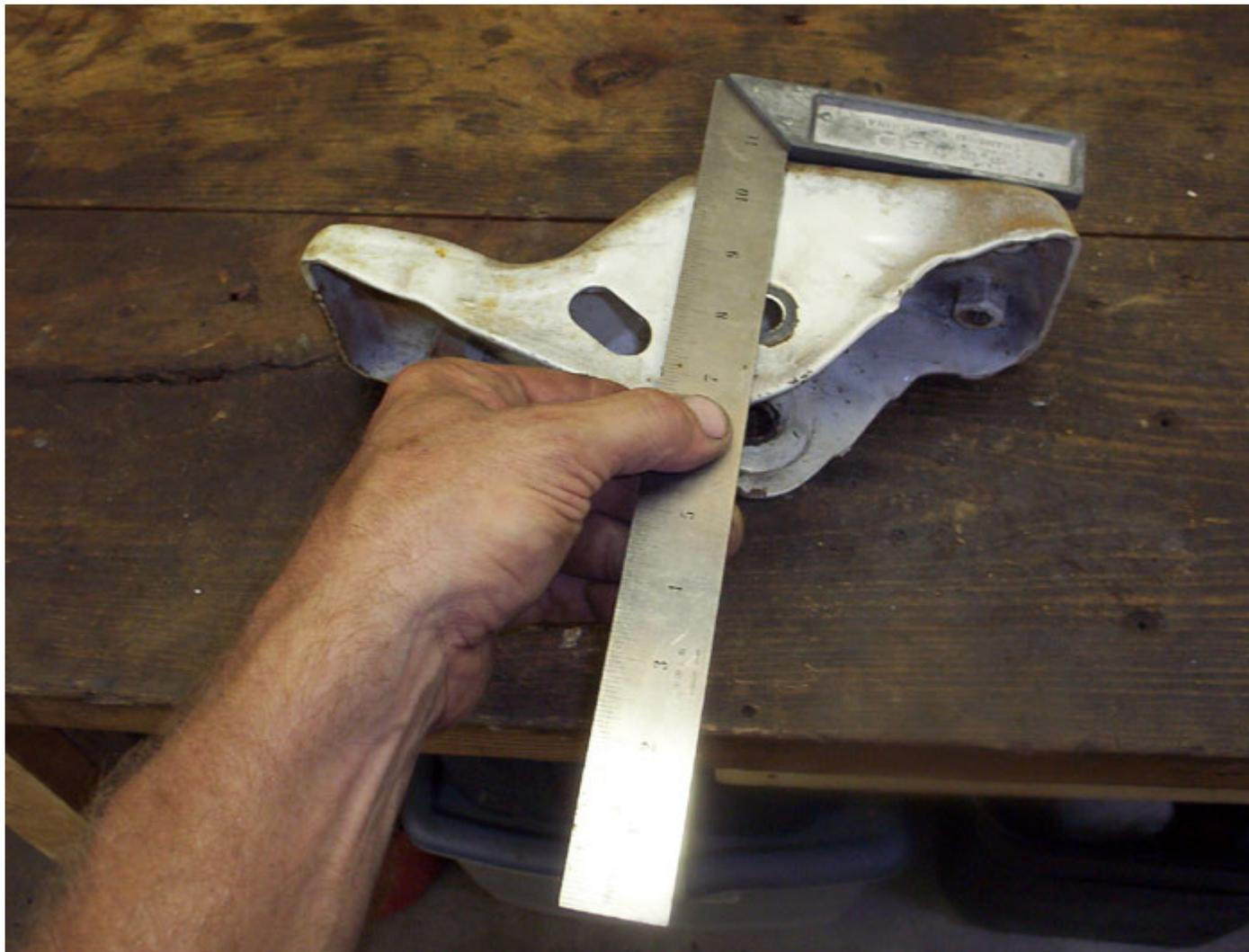
Here's the mounts with the new holes drilled, sandblasted and painted.
