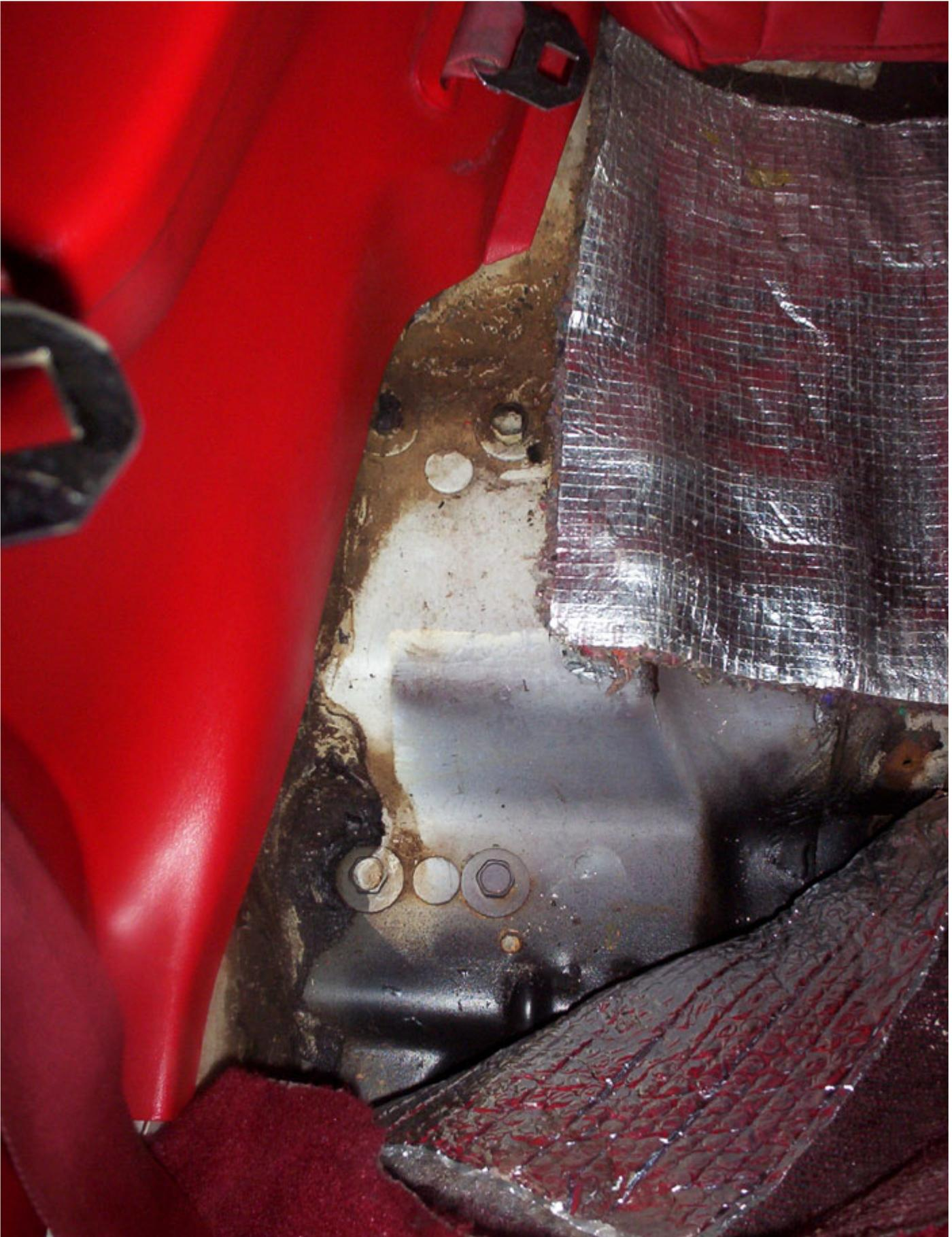
Here I am marking the mount for the new eye bolt holes. I scribed a line all the way to the top of the mount from the bolt centerline. Then I measured from the center of the rear unibody mounting holes to the eye bolt centerline. These measurements were the same on both
