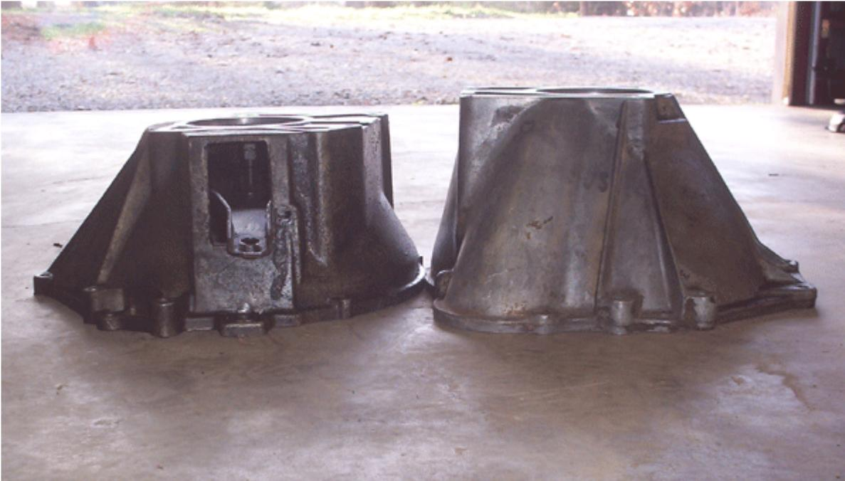
Here's the measurement of the fox body t-5 bell - just a little less than 7".
