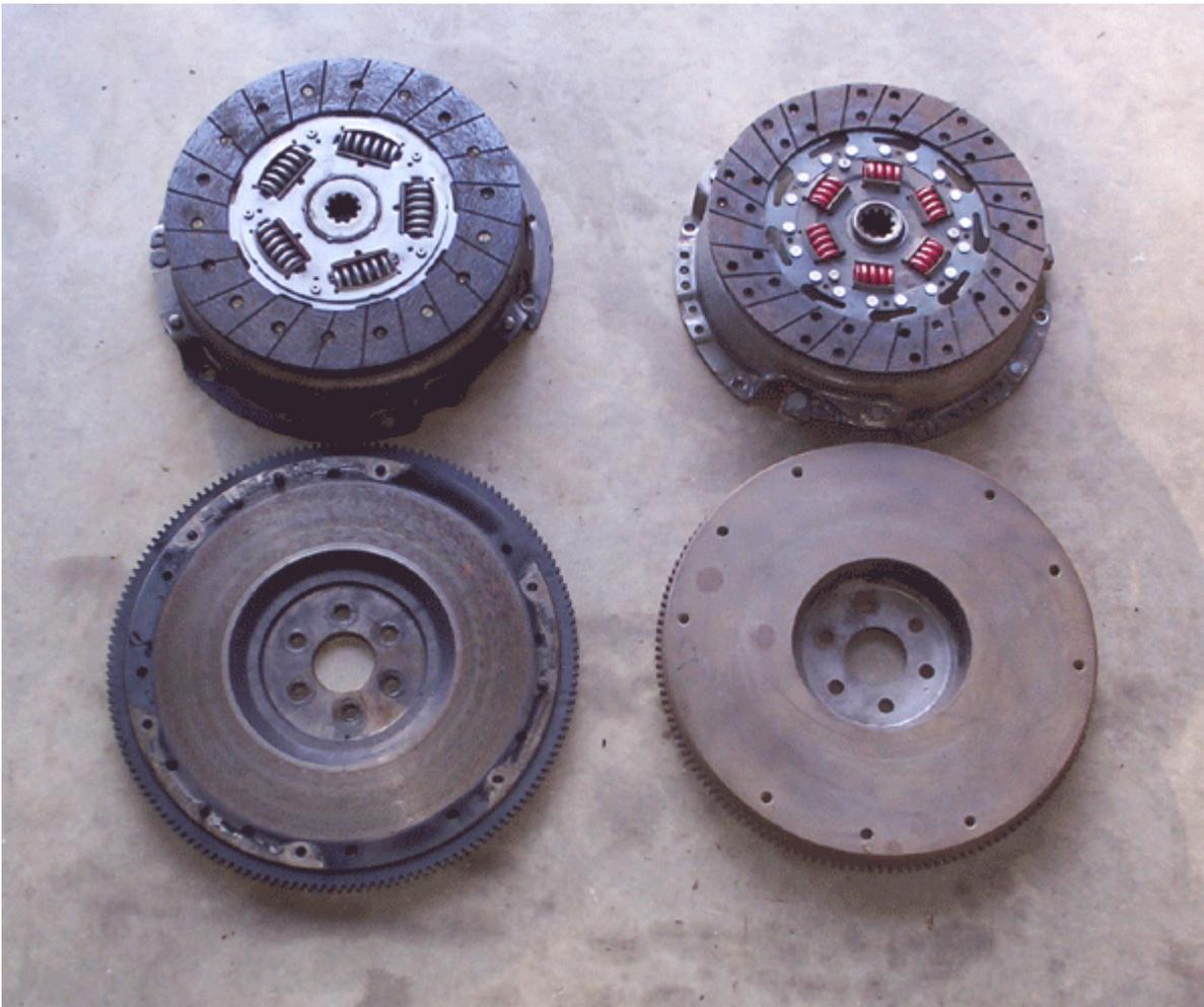
And here's the clutch disc comparison. The fox body t-5 clutch/pressure plate is 10.5 inches, the Mustang II clutch/pressure plate is 10".
