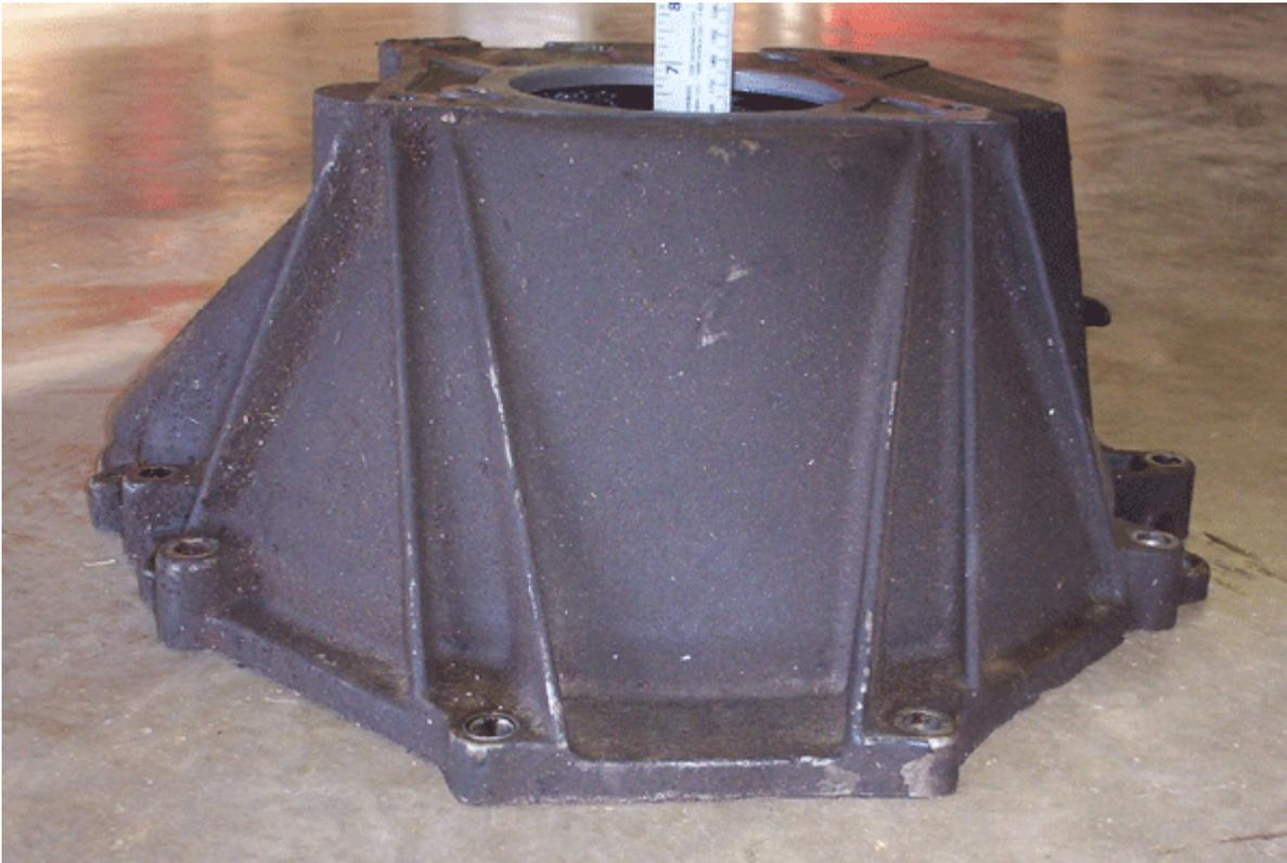
And here's the measurement of the v-8 Mustang II bell - just a little over 8".
