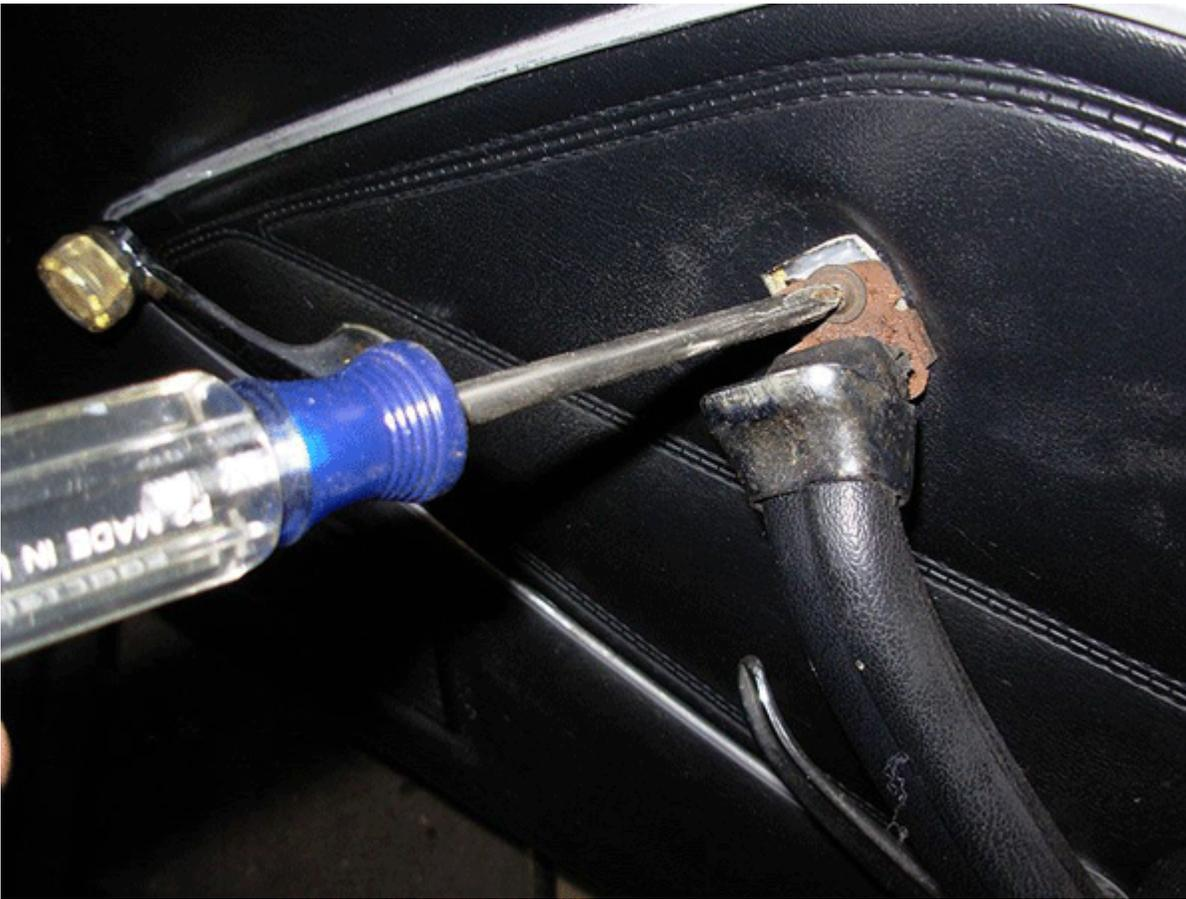
Remove the two 3/8 bolts that hold on the arm rest and the one Phillips screw located under the metal collar at the top of the arm rest. (The 1976 Cobra II arm rests are part of the door panel and do not need to be removed)
