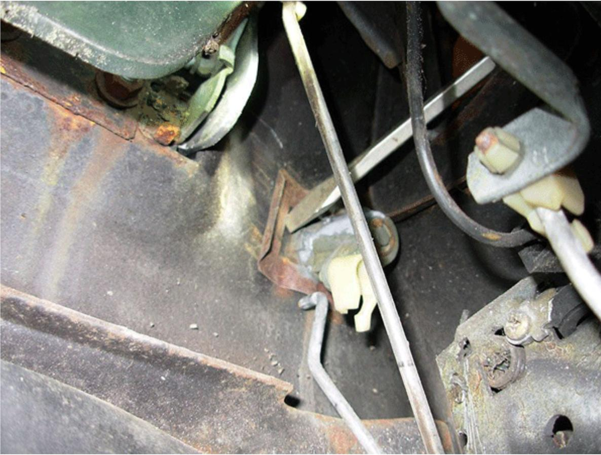
The metal clip can be removed with a long flat tip screwdriver by prying between the clip and the lock.
