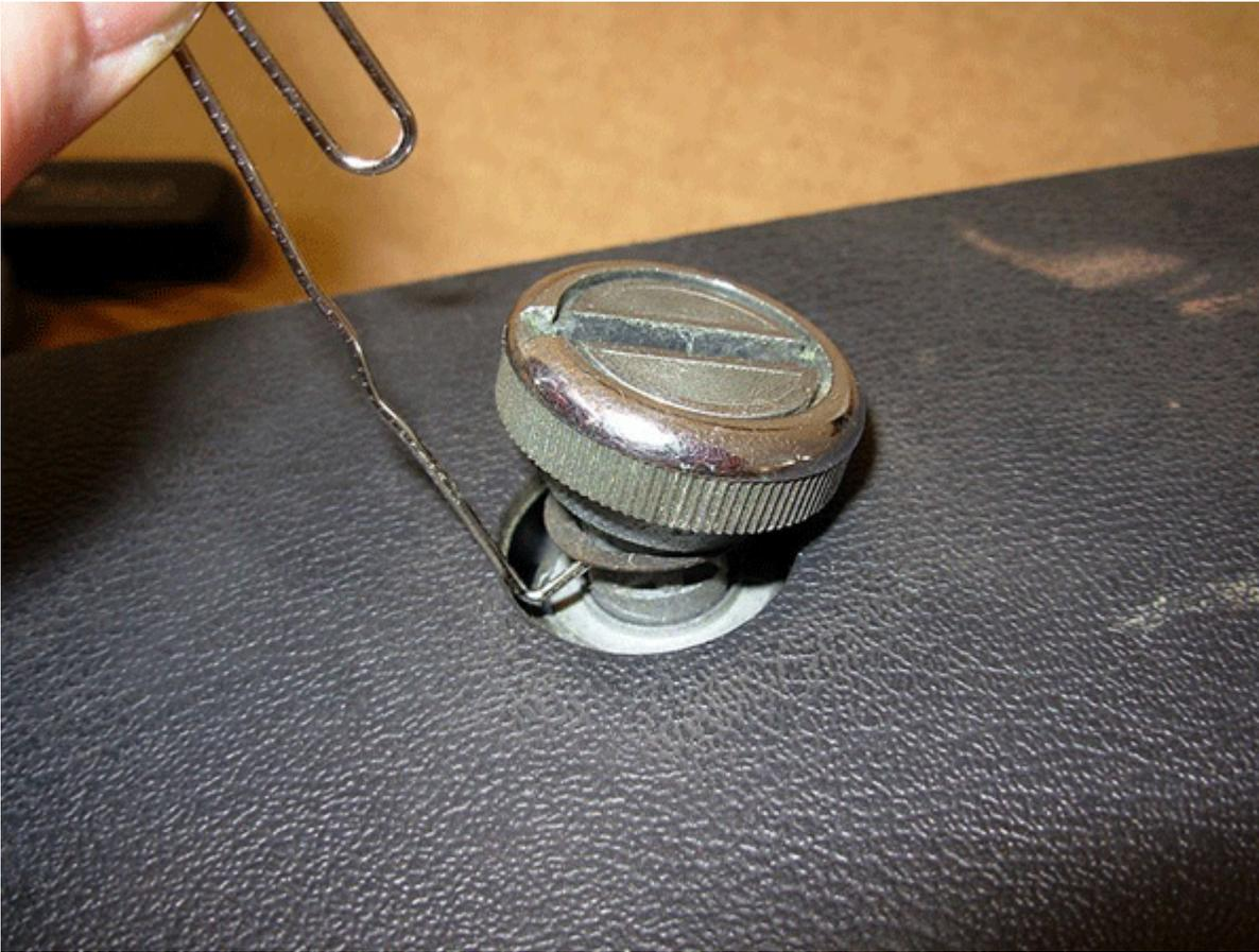
The door knob is just pressed on and held tight with a metal spring clip. Use a paper clip or pick to pull the clip towards the front of the knob to release it.
