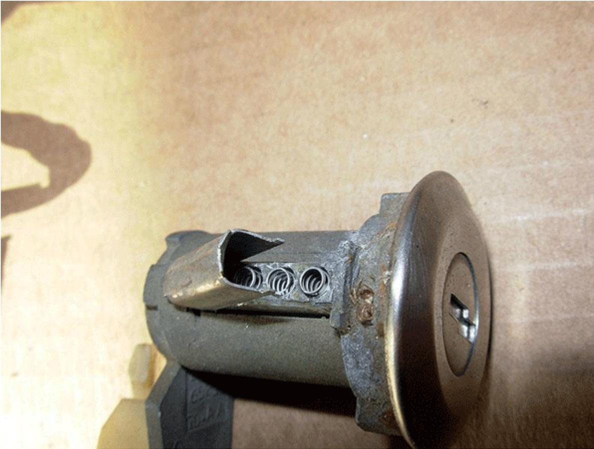
Slowly remove the metal cover on the side of the door lock by prying up on the front or back with a small screw driver or pick.
