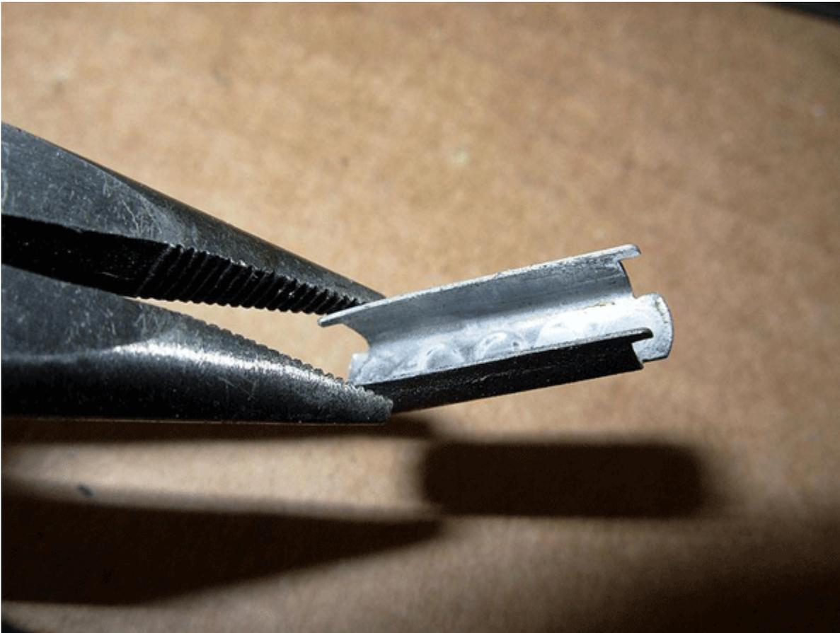
Lightly crimp the metal spring and pin cover and press it back into place.
