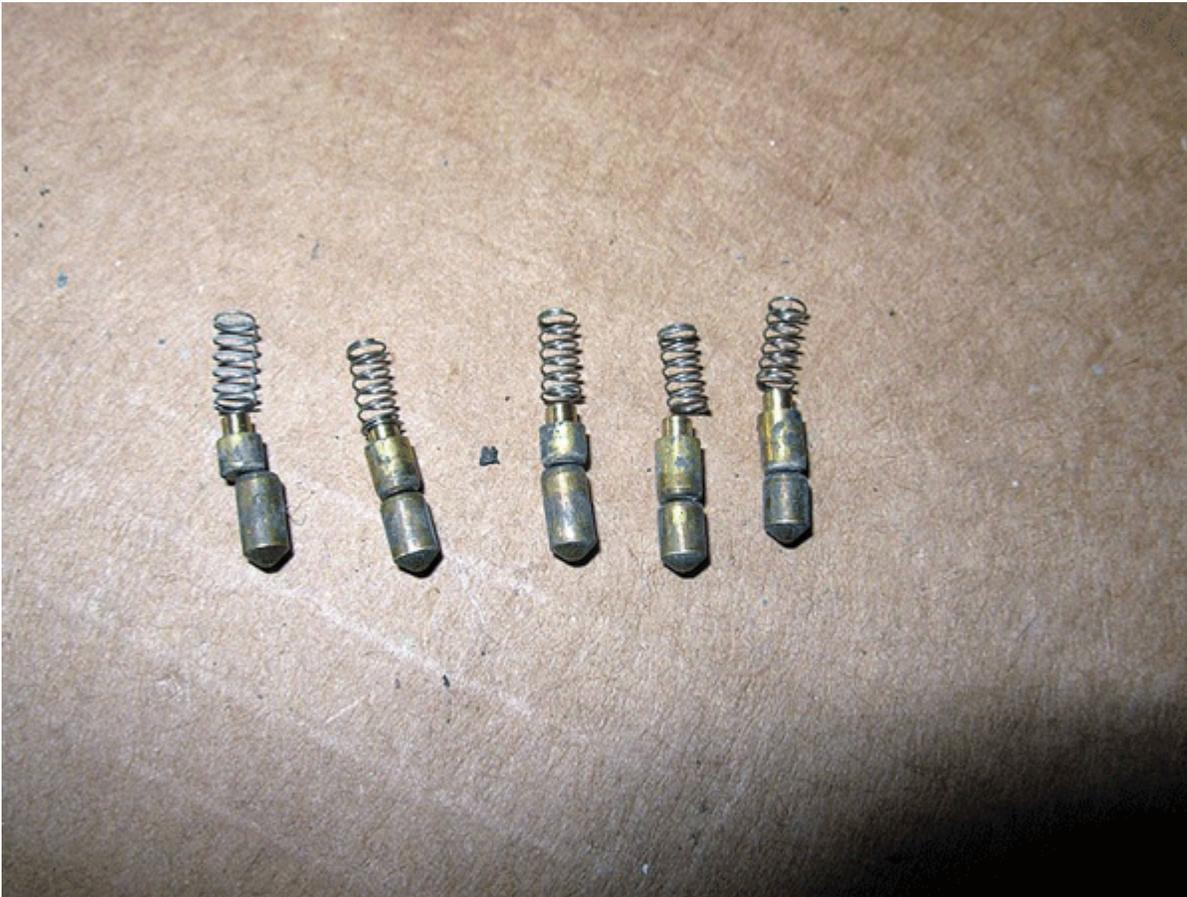
The pins with the points on them ride on the key, so the points always go into the cylinder holes first (pointing down).
