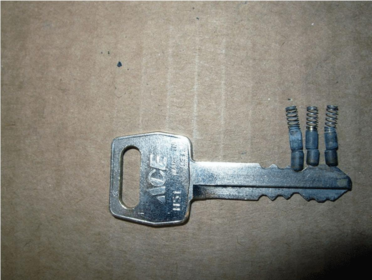
Notice how the lengths of the pins correspond to the depth of the cut in the key. The deeper the cut in the key, the longer the pin.
