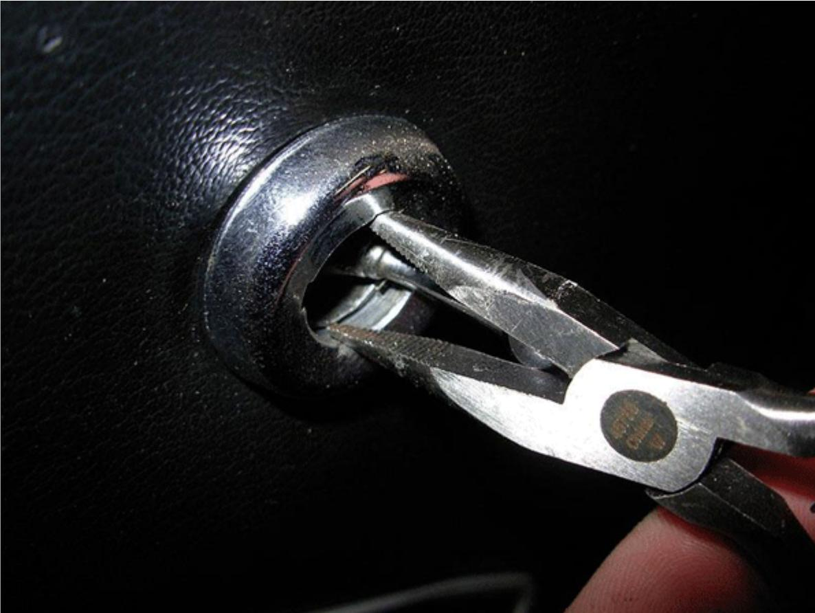
Remove the remote mirror bezel with a bezel removal tool or with a pair of needle nose pliers.
