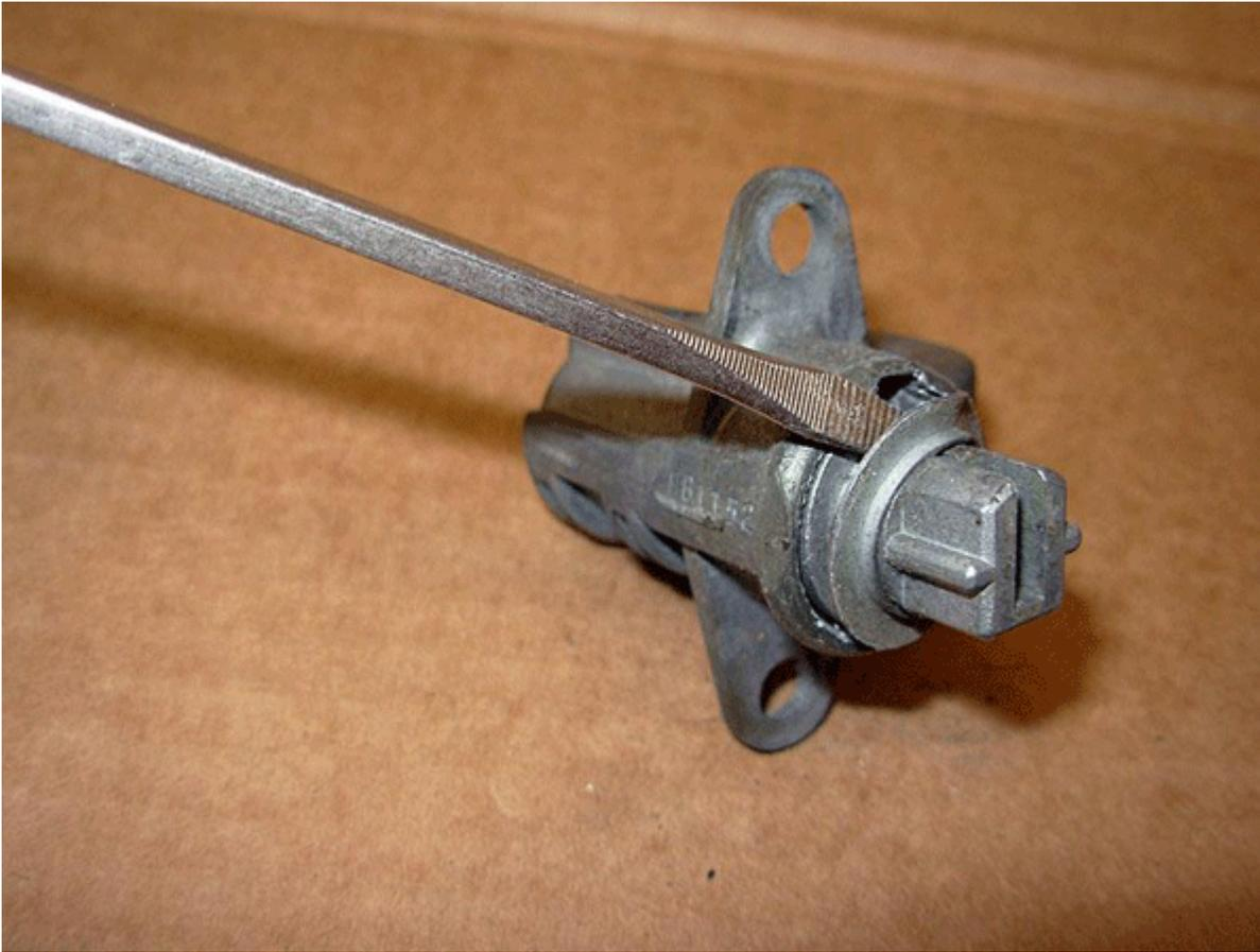
Once the washer is removed, pull out the lock cylinder from the glove box latch.
