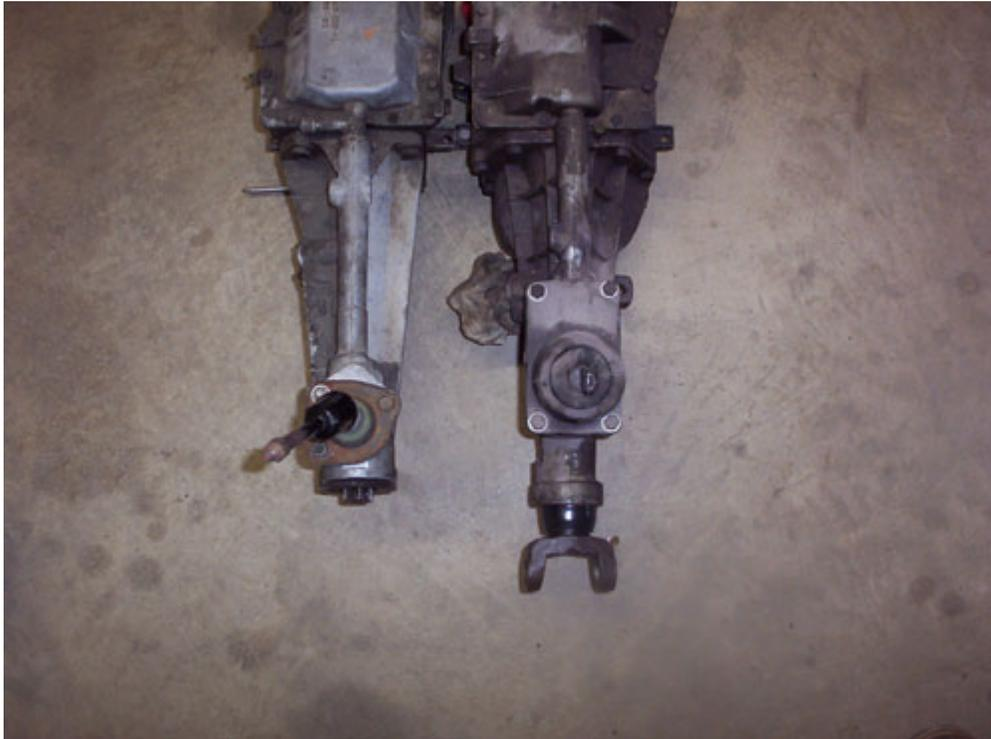
This pic shows the difference between crossmember mount location and the length of the input shaft. The T-5 is the lower one in the pic. This is an '84 T-5 and the 83-93 T-5 has an input that is about 1 1/4" shorter than the RAD. The 94-95 T-5 input shaft is about 3/4" longer than the 83-93 but still not quite as long as the RAD.
