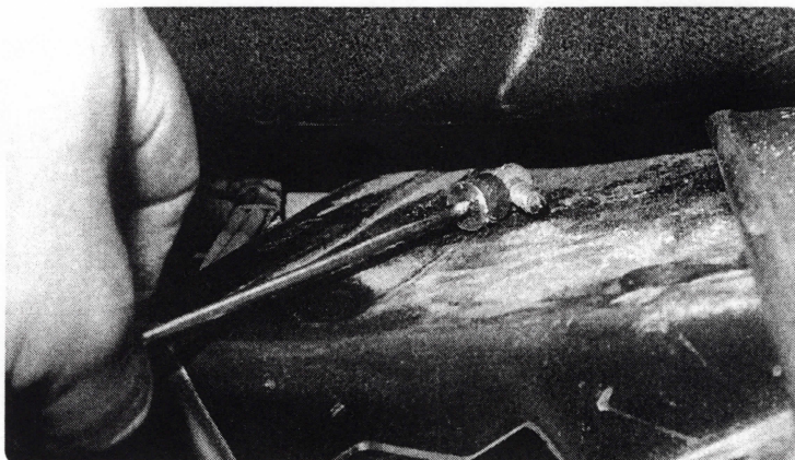
Pry down on the heater box assembly and use a magnet to retrieve that blasted screw.
