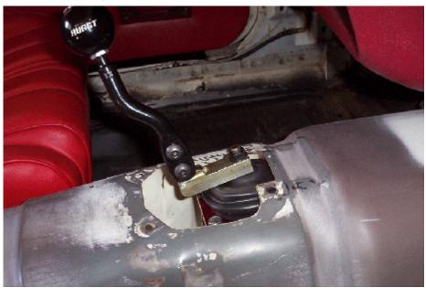
Here's a pic of the measurement from the tunnel to the center of the tailshaft on the t-5 to compare the position of the back of the trans to the RAD's position to make sure I didn't alter the driveshaft angle too much. The RAD tailshaft center was about 5" from the bottom of the tunnel and the t-5 is about 5 1/2". The 1/2" difference wasn't enough to set up a vibration from altering the angles.
