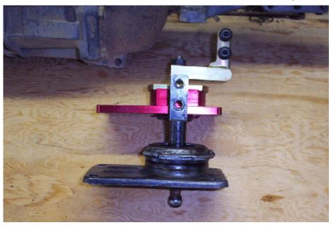
Here's a pic of the initial install with the trans in 4th gear. Notice the shifter is still a little too far forward and would hit the tunnel in 1st, 3rd or 5th. It's also very close to the bottom of the tunnel.
