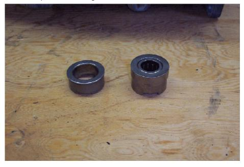
You will have to turn down the outside diameter of the input bearing retainer about .010" to fit into the Mustang II bellhousing. You can also enlarge the hole in the bellhousing but this way allows me to be able to use the same bell if I went back to the RAD for some reason. Here's a pic of the retainer after being turned down at the machine shop.
