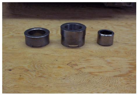
And here's a pic after the bearing was installed in the new sleeve.
