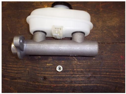
And here it is with the plug unsnapped from the reservoir. The sensor just snaps back in to reinstall, should I ever need to.
