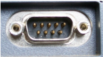
Standard DB9 male connector on computer.
