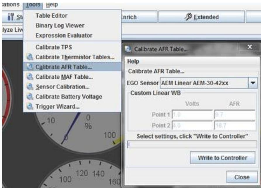
If you are using any non-Ford sensors (namely ACT/IAT or coolant temp), you'll need to calibrate them. Select (*Tools > Calibrate Thermistor Tables*). Most common options are available in the drop down menu. Click "Write to Controller" to finish the calibration.
