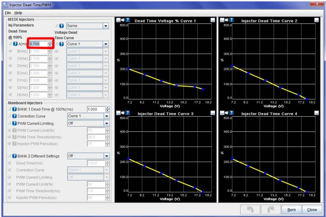
For factory 2.3T injectors, or Bosch & Delphi Low Imp, use 1.1. For TFX Low Imp, use 1.2. For factory V8 injectors use 0.9, for the High Imp Siemens Deka 4 Motron injectors we sell, use 0.8. If your injectors were supplied with dead time information such as our FID injectors, use your injector manufacturer data. More complete injector listing and additional details found in the 6<sup>th</sup> post of the FAQ here: [PiMPxs Injector Characteristics](#)
