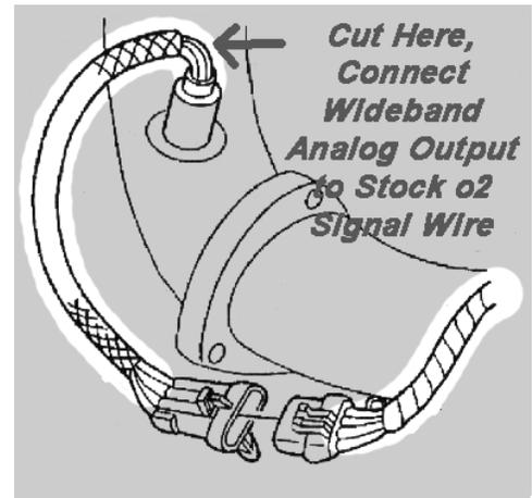
Just to be sure, it's best to test this with a multimeter to verify the wires you're trying to use have continuity to the right pin or are keyed power, ground, etc. If your colors don't match then you'll have to do this as there is no other way to ensure proper connection.
