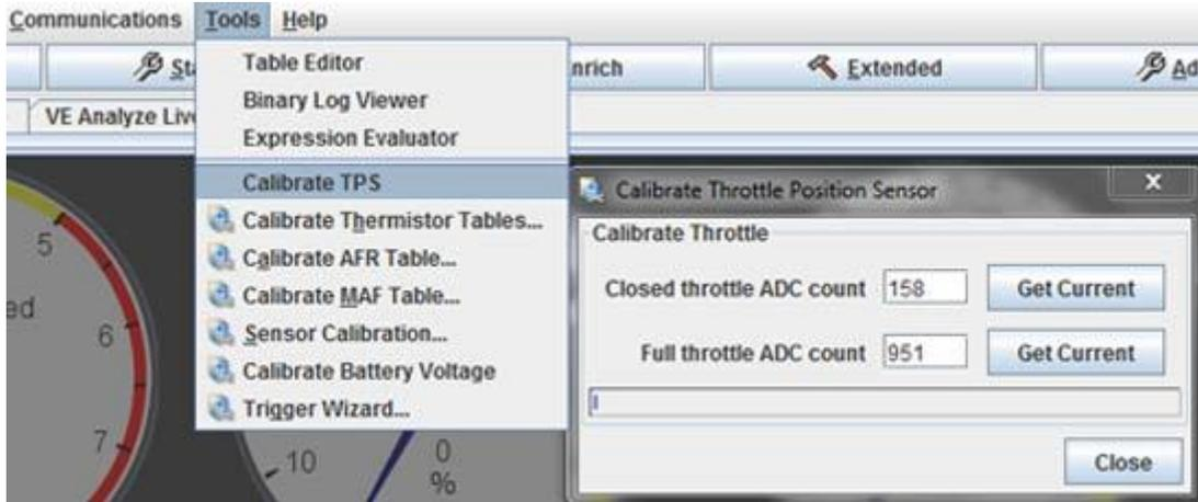
Wideband Sensor Calibration: select (*Tools > Calibrate AFR Table*) and then select the type of wideband sensor you are using. To ensure accurate calibration so your AFR reading in TunerStudio matches your wideband gauge, rather than selecting a pre-defined wideband option, instead select “Custom Linear WB” and enter the values in the table that match the settings your controller is using (found in the wideband instructions, listed as voltage vs AFR). Click “Write to Controller”.
