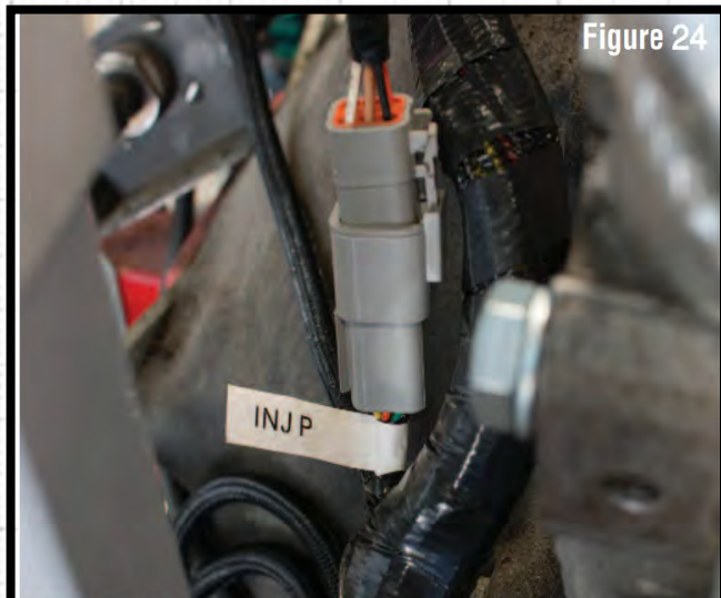
Figure 24 Injector P: This connector mates with the injector harness on the passenger side of the intake manifold.
