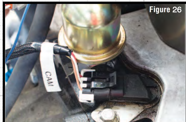
Figure 26 CAM: (LS1/LS6 shown)The cam position sensor of LS engines has changed throughout the years. Not only its location, but its wiring as well. Early models have the cam sensor located at the back of the block near the deck surface. During 2005, as a running change, the location changed to the front of the block between the cam and crankshaft. Must Used GM# 12627501.
