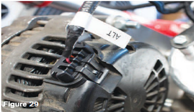
ALT: This wire directly connects to the alternator.
